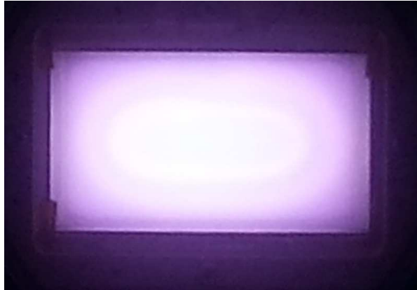
Figure 6.31: Picture of the PEGASES thruster without grids and magnets in a Xe discharge of 150 W.
