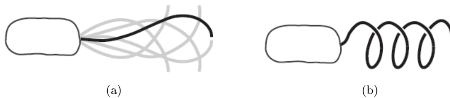
Figure 1.4: Two techniques to generate non-reciprocal motion: (a) The flexible oar oscillation: flagella create patterns such as traveling waves. (b) The corkscrew-type rotating propulsion: a molecular motor spins passive bacterial flagella [Abbott 2009].
