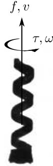
Figure 2.22: Upward direction is defined as the positive direction for f and v , the rotation direction in which SHM1-mh8 rotates to generate a positive force is defined as the positive direction for \tau and \omega .
