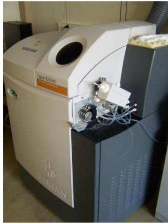
Figure II-19 : Appareillage ICP/MS VARIAN 810-820-MS
