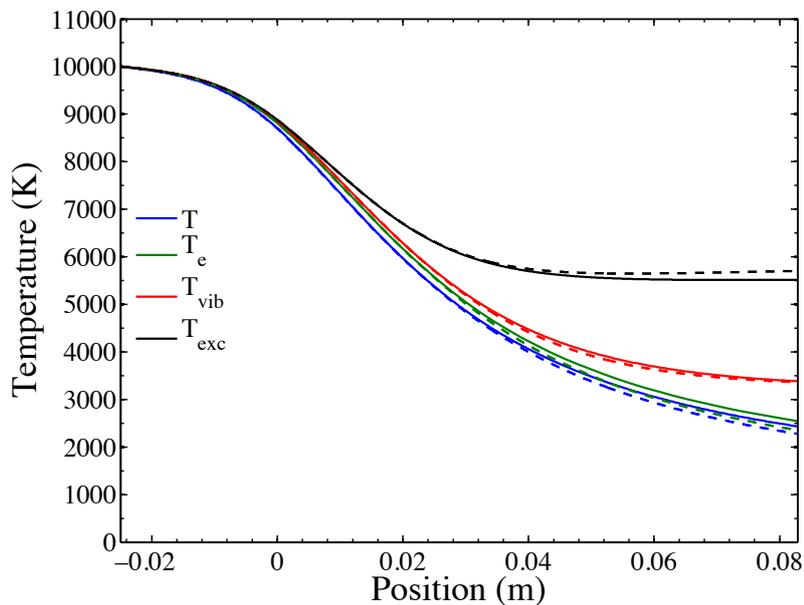
**Figure 7.29:** Evolution of translation temperature  $T$ , electron temperature  $T_e$ ,  $N$  electronic temperature  $T_{exc}$  and vibrational temperature  $T_{vib}$  along the nozzle axis. Optically thick (solid) and coupled (dashed) results. Test case C.
