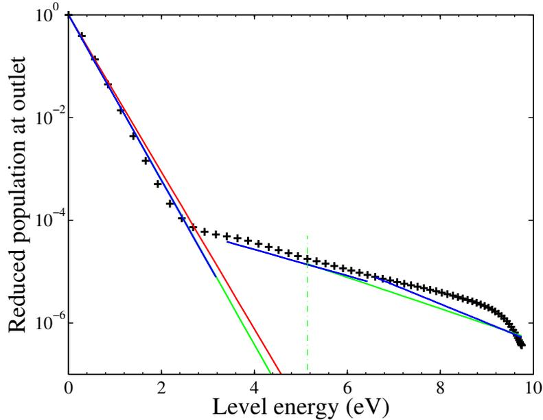
**Figure 8.26:** *Vibrational distribution functions at the nozzle outlet with the detailed model (crosses), with the 1Tv – StSRed model (red), with the 2Tv – StSRed model (green) and with the 3Tv – StSRed model (blue). Test case A of table 7.1.*
