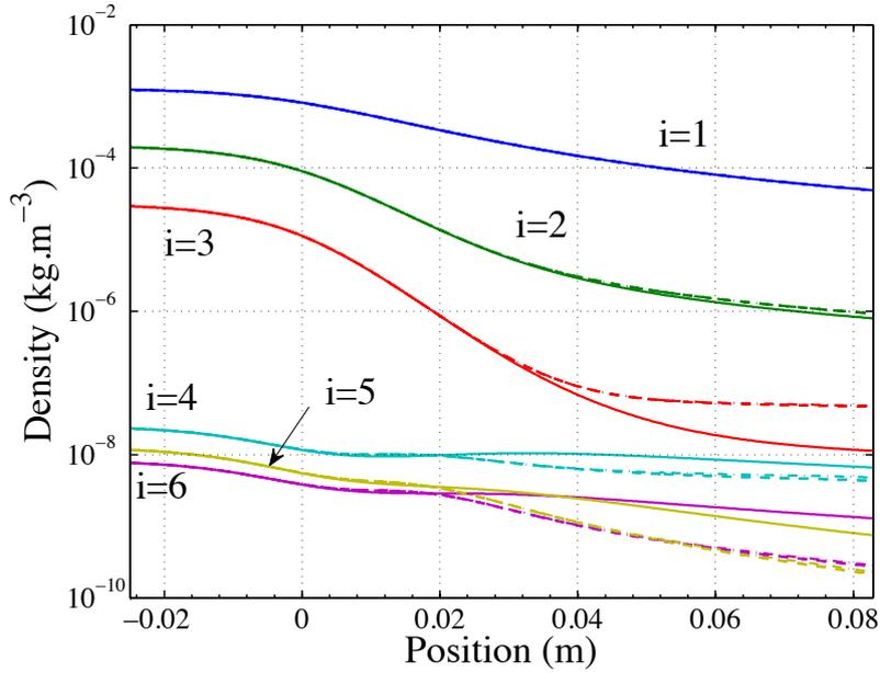
**Figure 7.32:** Evolution of the densities of the six lowest levels of  $N$  for the optically thick calculation (solid) and for the coupled calculations after 74 iterations (dash-dotted) and after 115 iterations (dashed). Test case  $C$
