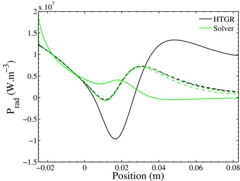
**Figure 7.27:** Evolution of  $P_{rad}$  along the nozzle axis computed by the flow solver (green) and by HTGR (black). Results for the first iteration (solid), and for the iterations 52 (dash-dotted) and 115 (dashed). Test case C.
