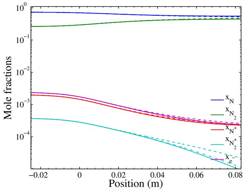
**Figure 8.28:** Evolution of compositions along the nozzle axis predicted with the detailed model (solid), with the  $1Tv - StSRed$  model (dashed), the  $2Tv - StSRed$  model (dash-dotted) and the  $3Tv - StSRed$  model (dotted). Test case B of table 7.1.
