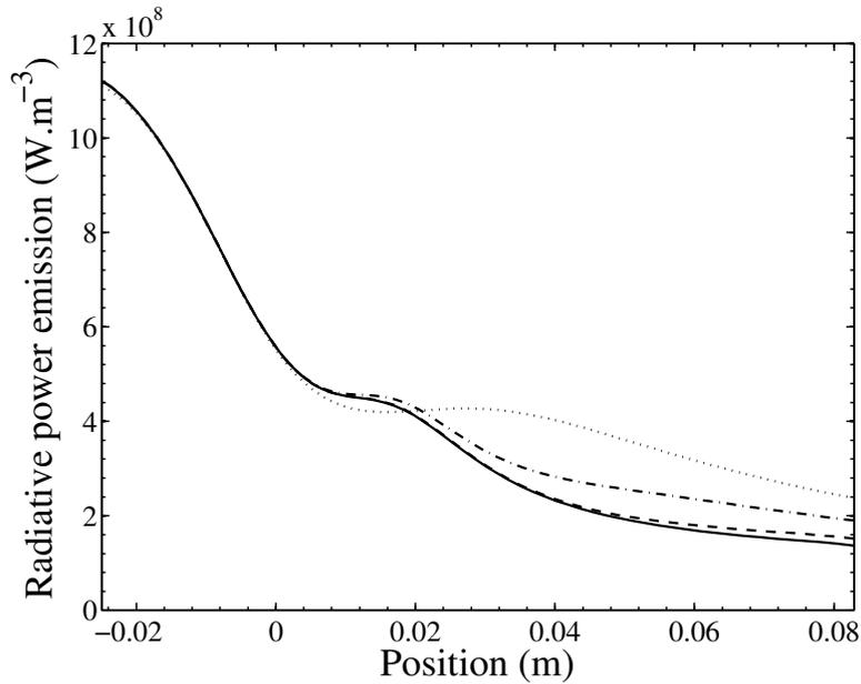
**Figure 7.28:** Evolution of the emission power along the nozzle axis computed by HTGR. Results for the first iteration (dotted), after 22 (dash-dotted), 74 (dashed) and 115 (solid) iterations. Test case C.
