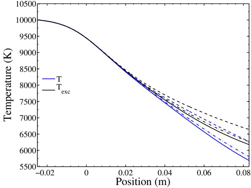
**Figure 8.27:** Evolution of temperatures along the nozzle axis predicted with the detailed model (solid), with the  $1Tv - StSRed$  model (dashed), the  $2Tv - StSRed$  model (dash-dotted) and the  $3Tv - StSRed$  model (dotted). Test case B of table 7.1.
