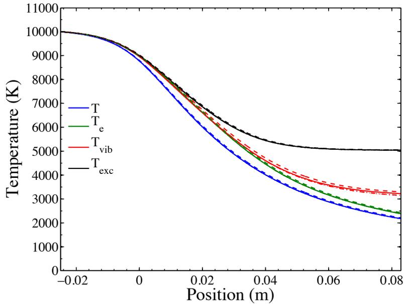
**Figure 8.24:** Evolution of temperatures along the nozzle axis predicted with the detailed model (solid), with the  $1Tv - StSRed$  model (dashed), the  $2Tv - StSRed$  model (dash-dotted) and the  $3Tv - StSRed$  model (dotted). Test case A of table 7.1.
