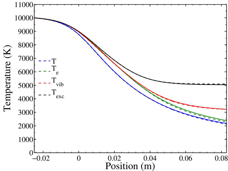
**Figure 7.34:** Evolution of translation temperature  $T$ , electron temperature  $T_e$ ,  $N$  electronic temperature  $T_{exc}$  and vibrational temperature  $T_{vib}$  along the nozzle axis. Optically thick (solid) and coupled (dashed) results. Test case A.
