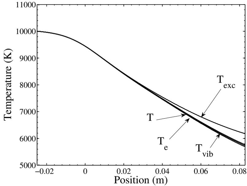
**Figure 7.14:** Evolution of translation temperature  $T$ , electron temperature  $T_e$ ,  $N$  electronic temperature  $T_{exc}$  and vibrational temperature  $T_{vib}$  along the nozzle axis. Case B of table 7.1 with the model II of table 7.5.
