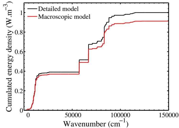
**Figure A.10:** Cumulated radiative energy density at  $x = 0.46$  cm behind the shock wave, normalized by the results of the detailed model. Results of the detailed (black line) and of the macroscopic (red lines) models for electronic excitation. Fire II 1634s test case.
