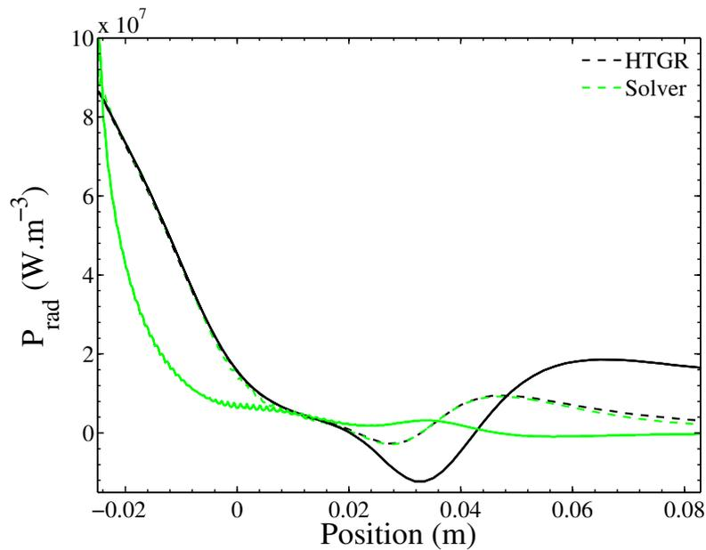
**Figure 7.33:** Evolution of  $P_{rad}$  along the nozzle axis computed by the flow solver (green) and by HTGR (black). Results for the first iteration (solid), and after 74 iterations (dashed). Test case  $A$ .
