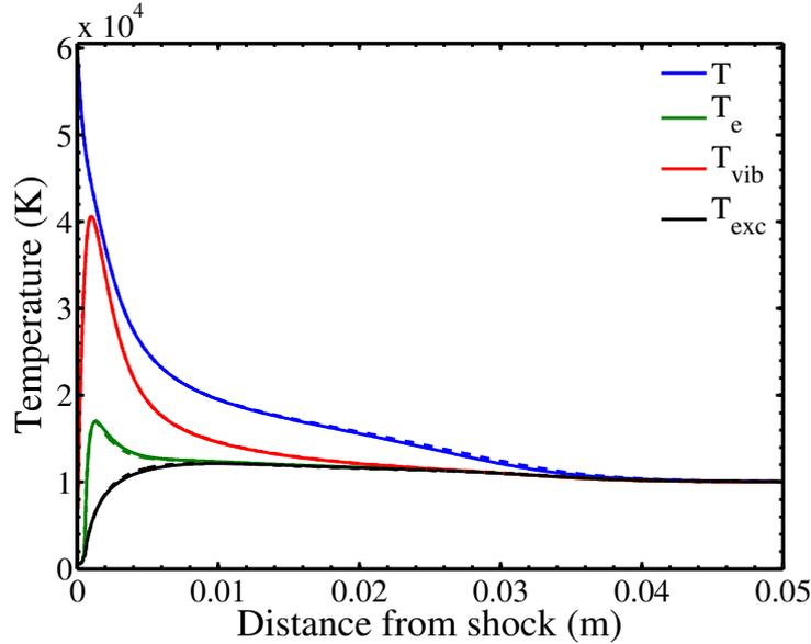
**Figure A.1:** Evolution of temperatures behind the shock wave obtained with the detailed model (solid) and with the macroscopic model (dashed) for electronic excitation. Fire II 1634s test case.
