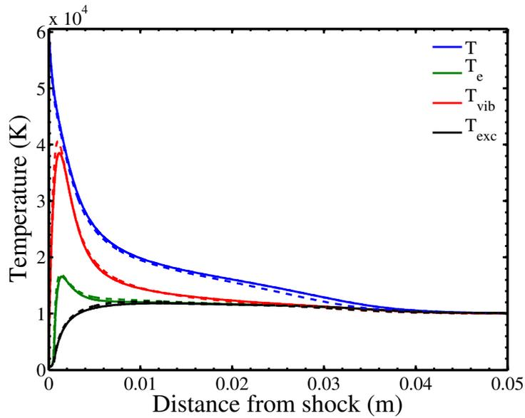
**Figure 8.2:** Evolution of temperatures behind the shock wave with the detailed model (solid) and with the  $1Tv - StSRed$  model (dashed). Fire II 1634s test case.
