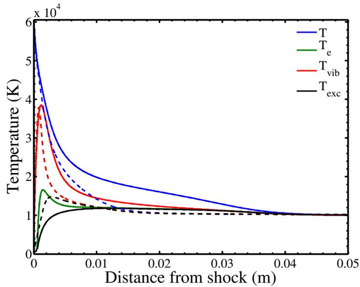
**Figure 8.7:** Evolution of temperatures behind the shock wave with the detailed model (solid) and with the  $T_{ve}$  model (dashed). Fire II 1634s test case.
