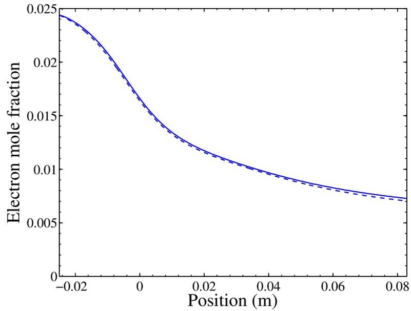
**Figure 7.35:** Evolution of electron mole fraction along the nozzle axis. Optically thick (solid) and coupled (dashed) results. Test case A.
