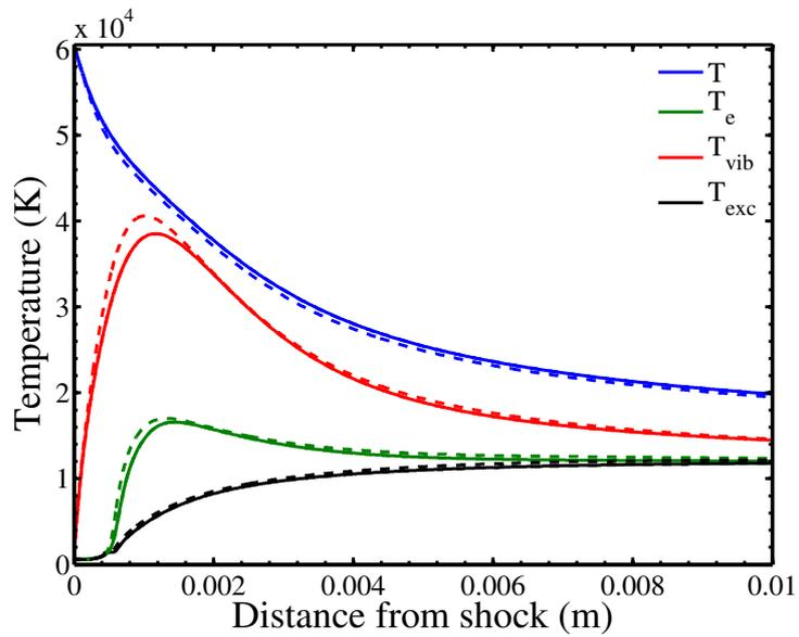
**Figure 8.3:** Evolution of temperatures behind the shock wave with the detailed model (solid) and with the  $1Tv - StSRed$  model (dashed). Zoom just behind the shock wave. Fire II 1634s test case.
