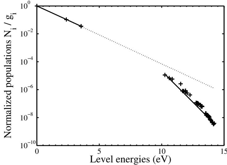
**Figure A.6:** Nitrogen atom electronic states populations divided by their degeneracies at  $x = 1$  cm behind the shock obtained with the detailed model (symbols). Boltzmann distribution at the equivalent  $T_{exc}$  (dotted line), and 2-group distribution obtained with the macroscopic model for electronic excitation (solid lines). Fire II 1634s test case.
