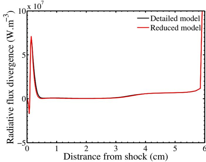
**Figure A.9:** Evolution of the radiative flux divergence behind the shock wave. Results of the detailed (black line) and of the macroscopic (red lines) models for electronic excitation. Fire II 1634s test case.
