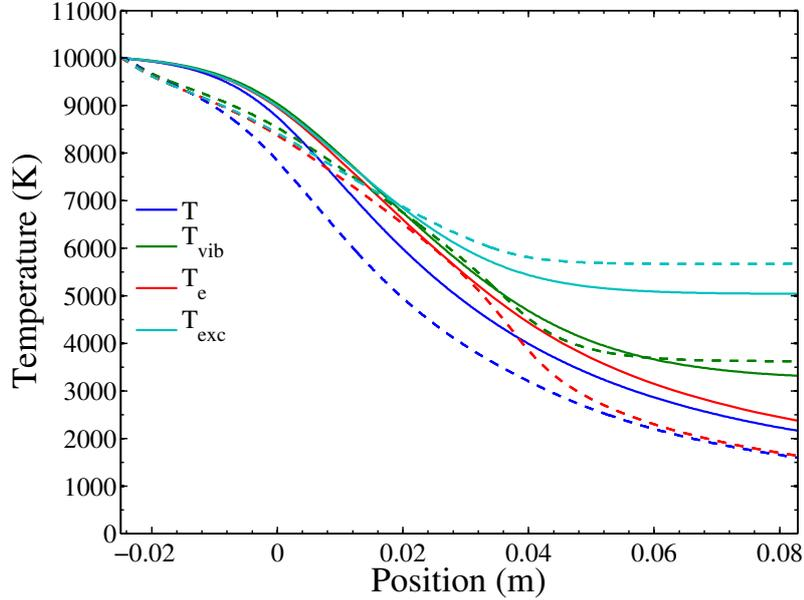
**Figure 7.23:** Evolution of translation temperature  $T$ , electron temperature  $T_e$ , excitation temperature  $T_{exc}$  and vibrational temperature  $T_{vib}$  along the nozzle axis. Comparison between optically thick (solid) and thin (dashed) assumptions. Test case A.
