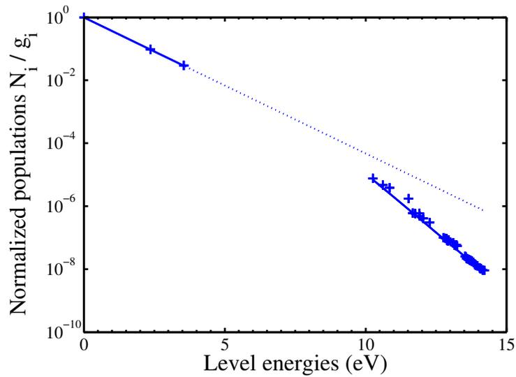
**Figure A.7:** Nitrogen atom electronic states populations divided by their degeneracies at  $x = 2$  cm behind the shock obtained with the detailed model (symbols). Boltzmann distribution at the equivalent  $T_{exc}$  (dotted line), and 2-group distribution obtained with the macroscopic model for electronic excitation (solid lines). Fire II 1634s test case.
