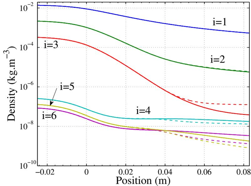
**Figure 7.37:** Evolution of the densities of the six lowest levels of  $N$  for the optically thick calculation (solid) and for the coupled calculations after 74 iterations (dash-dotted) and after 115 iterations (dashed). Test case A.
