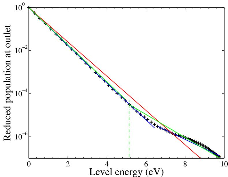
**Figure 8.29:** Evolution of compositions along the nozzle axis predicted with the detailed model (crosses), with the  $1Tv - StSRed$  model (red), with the  $2Tv - StSRed$  model (green) and with the  $3Tv - StSRed$  model (blue). Test case B of table 7.1.
