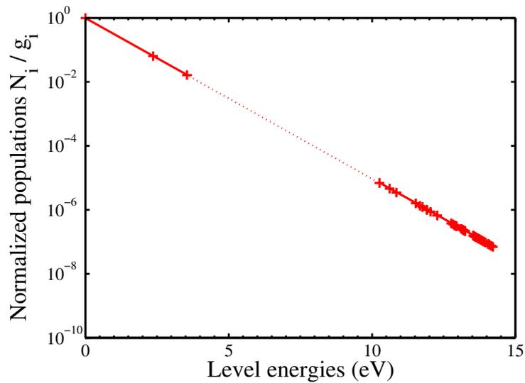
**Figure A.8:** Nitrogen atom electronic states populations divided by their degeneracies at  $x = 5$  cm behind the shock obtained with the detailed model (symbols). Boltzmann distribution at the equivalent  $T_{exc}$  (dotted line), and 2-group distribution obtained with the macroscopic model for electronic excitation (solid lines). Fire II 1634s test case.
