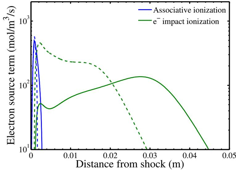
**Figure 8.15:** *Electron creation by associative ionization (blue) and electron impact ionization (green) with the 1Tv – StSRed model (solid) and with the MT model (dashed). Fire II 1634s test case.*
