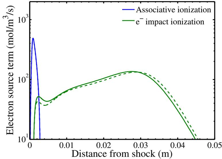
**Figure A.4:** *Electron creation by associative ionization (blue) and electron impact ionization (green) with the detailed model (solid) and with the macroscopic model (dashed) for electronic excitation. Fire II 1634s test case.*
