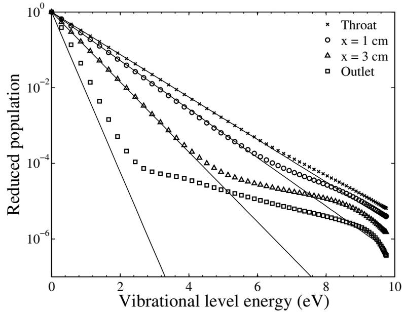
**Figure 7.12:** *Vibrational distribution function of  $N_2$  at 4 locations along the nozzle axis (symbols) and vibrational distribution functions at the electron temperature (lines). Case A of table 7.1 with the full model II of table 7.5.*
