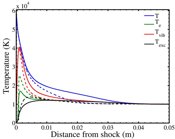
**Figure 8.12:** Evolution of temperatures behind the shock wave with the 1Tv–StSRed model (solid) and with the MT model (dashed). Fire II 1634s test case.
