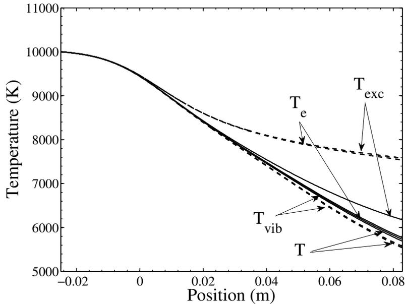
**Figure 7.20:** Evolution of translation temperature  $T$ , electron temperature  $T_e$ ,  $N$  electronic temperature  $T_{exc}$  and vibrational temperature  $T_{vib}$  along the nozzle axis. Case B of table 7.1, with (solid) and without (dashed)  $e - V$  processes.
