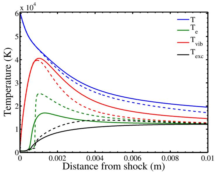
**Figure 8.13:** Evolution of temperatures behind the shock wave with the 1Tv–StSRed model (solid) and with the MT model (dashed). Zoom just after the shock. Fire II 1634s test case.
