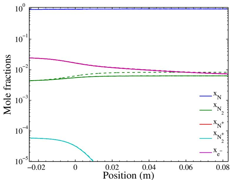
**Figure 8.25:** Evolution of compositions along the nozzle axis predicted with the detailed model (solid), with the  $1Tv - StSRed$  model (dashed), the  $2Tv - StSRed$  model (dash-dotted) and the  $3Tv - StSRed$  model (dotted). Test case A of table 7.1.
