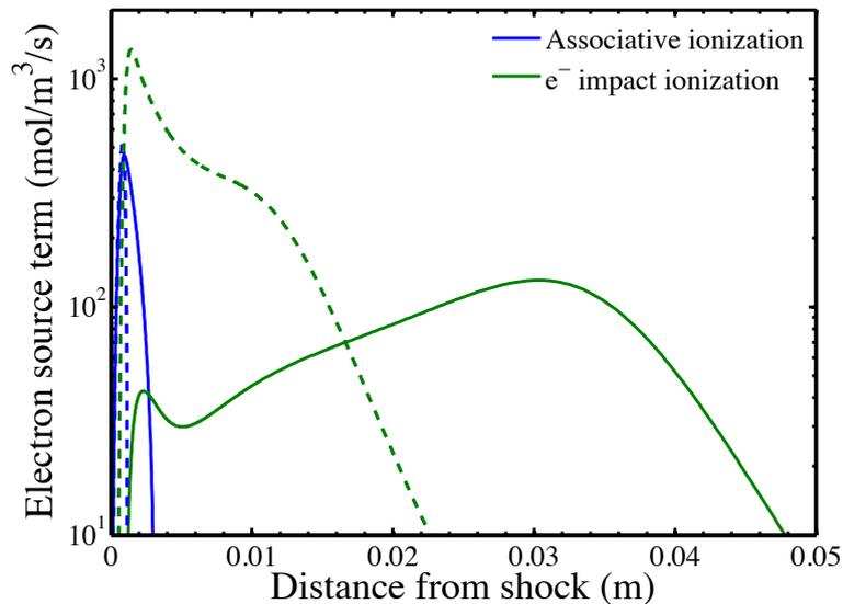
**Figure 8.10:** Electron creation by associative ionization (blue) and electron impact ionization (green) with the detailed model (solid) and with the  $T_{ve}$  model (dashed). Fire II 1634s test case.
