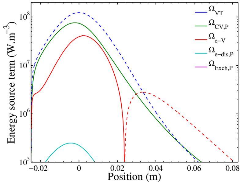
**Figure 7.11:** Evolution of vibrational energy creation terms (solid) and depletion terms (dashed) along the nozzle axis. Case A of table 7.1 with model II of table 7.5.
