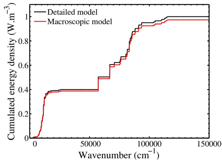
**Figure A.11:** Cumulated radiative energy density at  $x = 5.24$  cm behind the shock wave. Results of the detailed (black line) and of the macroscopic (red lines) models for electronic excitation. Fire II 1634s test case.
