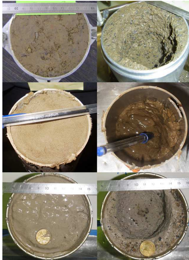
Figure 3.25. Photographs of soil samples before (left) and after (right) JETs, with from top to bottom images corresponding to soils A, B and C, respectively.
