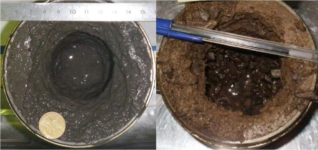
Figure 2.2. Illustration of standard erosion figures obtained following Jet Erosion Tests (C. Moras - geophyConsult).
