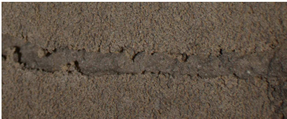
Figure 4.34. Illustration of typical profiles of scour holes obtained following the HET tests (F. Byron, IRSTEA).
