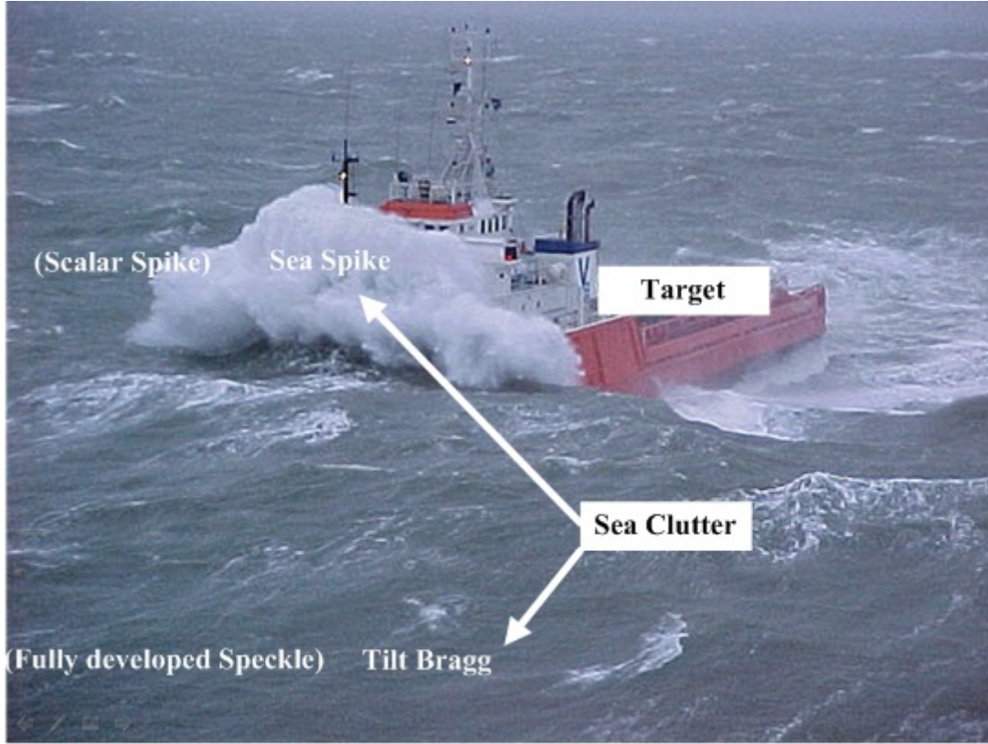
Figure 1.4 — Sea clutter and ship target (photo from internet)
