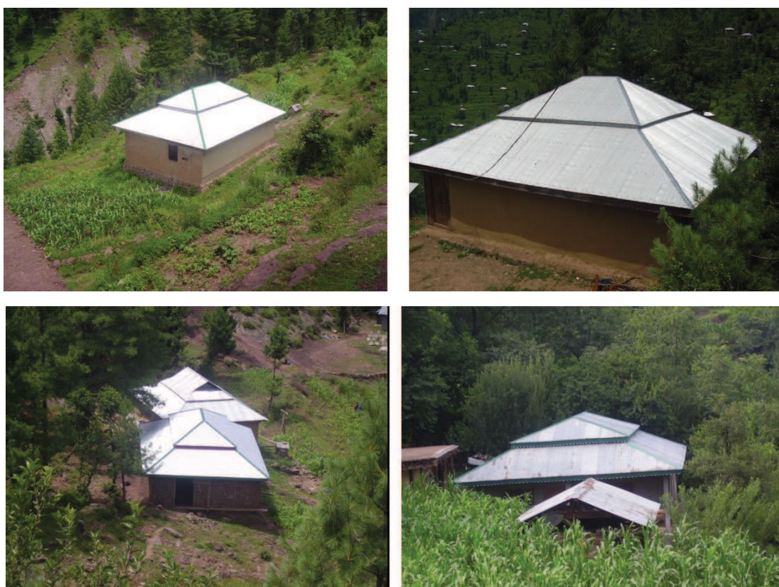
Figure 6.30 — Negligible break hip roof. Source : S. Abidi
