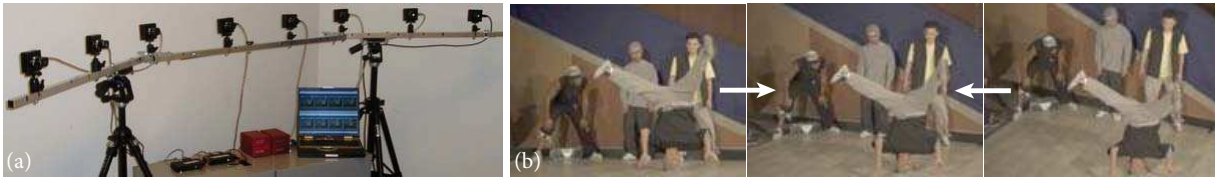
Figure 2.5: Joint stereo and image-based rendering. (a) Studio capture setup used in Zitnick et al. [2004]; Zitnick and Kang [2007]. (b) Input images are shown on left and right and interpolated view shown in the middle. These approaches are limited to view interpolation over fairly small baselines.
