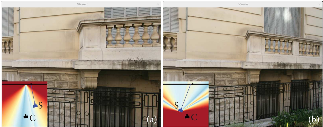
Figure 5.10: Interactive navigation tool. (a) When the user translates, the inset shows predicted ratings for all camera positions keeping the orientation fixed. (b) When the user turns, the inset shows ratings for all possible camera orientations keeping the position fixed. The application restricts the user navigation to regions with acceptable predicted quality. Capture camera is indicated by “C”, simulation camera by “S”, façade by a black line and corner by a black dot on the black line in the insets.
