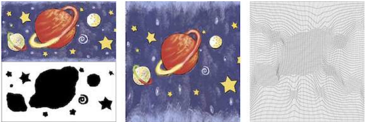
Figure 2.7: Variational warps [Gal et al. , 2006] for retargeting. The input image (upper left) is warped to produce the result (middle). The saliency mask (lower left) is used to impose constraints on the vertices of a regular warp mesh, which get deformed to the final underlying warp mesh shown on the right.
