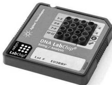
Figure 3: This chip is commercialized by Agilent Technologies and permits the identification of specific genetic sequences in a 1\text{-}\mu\text{l} sample of roughly purified DNA. The process time is just about 10 min [1].
