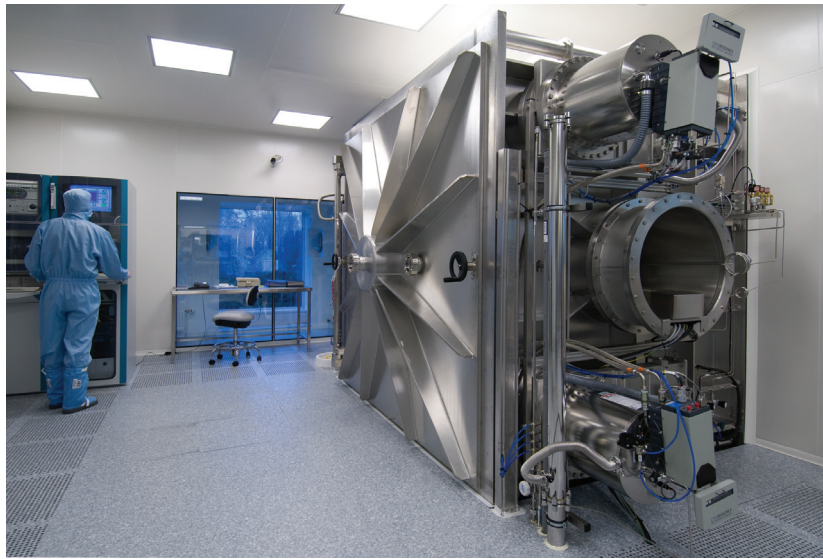
Figure 6.4: The large Ion Beam Sputtering coating machine.
