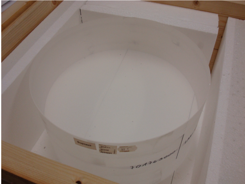
Figure 1.12: Input mirror blank (35 cm diameter, 20 cm thickness).
