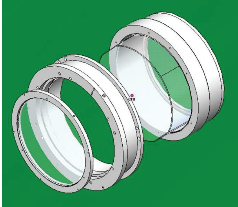
Figure 4.3: Exploded view of the sample holder for the measurement of aLIGO mirror surface figures with phase-shifting interferometry. The tested surface is located on the right of the figure. Plexiglass allows to protect the substrate surfaces while being handled.
