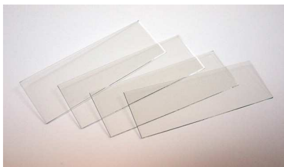
Figure 6.8: ITO plates used in our study
