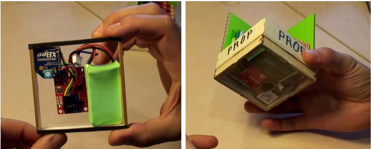
Figure 5.9: The tracker unit that attaches to the bottom of a physical bar chart.
