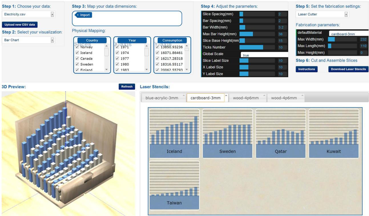
**Figure 7.7:** Overview of the MakerVis user interface. The steps involved in the workflow are grouped horizontally on the top with previews of the results, here 3D assembly and laser stencil preview, being placed below.
