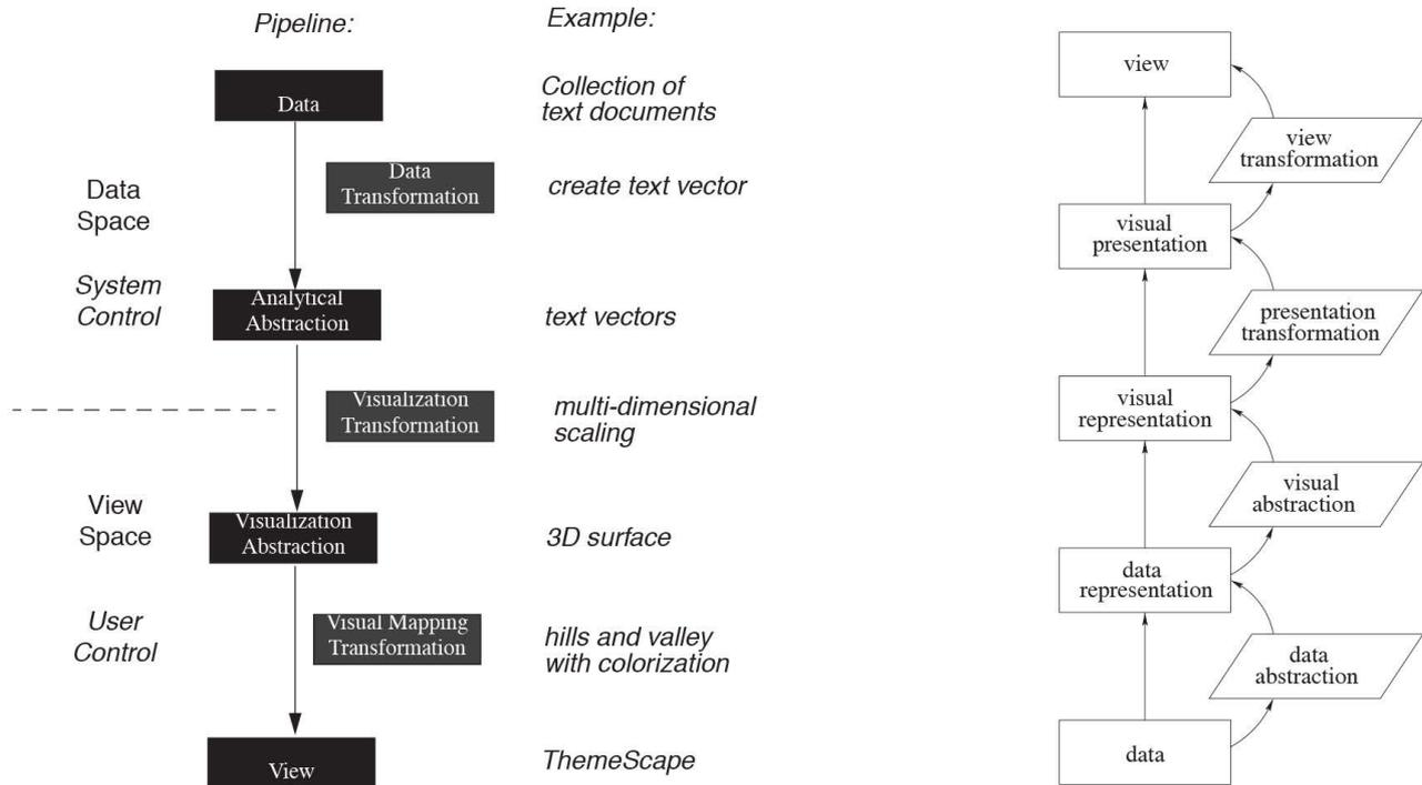
**Figure 6.2:** Left: the operator interaction framework (to be read from top to bottom) by Chi and Riedl [CHI AND RIEDL, 1998]. Right: pipeline introducing the presentation space (to be read from bottom to top) by Carpendale [1999]
