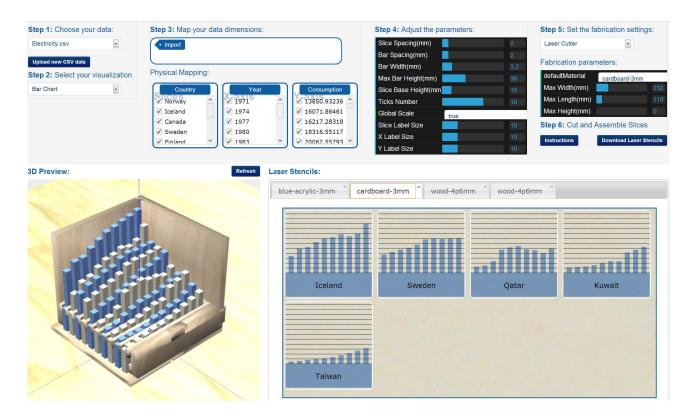
**Figure 7.7:** Overview of the MakerVis user interface. The steps involved in the workflow are grouped horizontally on the top with previews of the results, here 3D assembly and laser stencil preview, being placed below.
