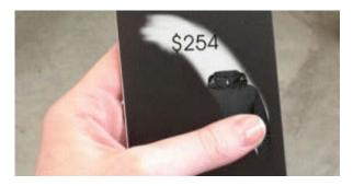
**Figure 8.7:** The exact value of data point can be revealed by touching a surface covered with thermochromic ink while otherwise reducing visual clutter by hiding such details.
