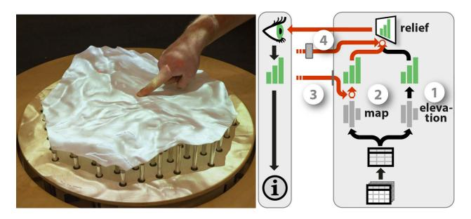
Figure 6.27: Direct interaction with topographic data using Relief [Leithinger et al., 2011].
