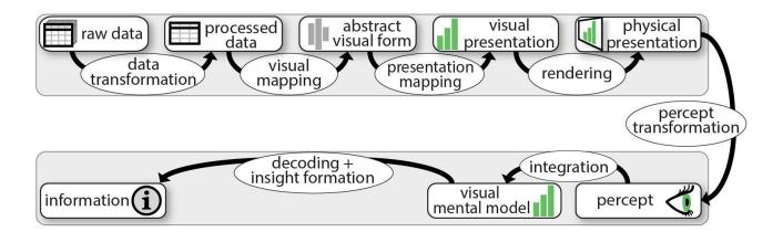
**Figure 6.3:** Our extended version of the infovis pipeline. The visualization system is on the top and reads left to right as in [CARD ET AL., 1999]. The user is depicted underneath. User interactions can take place on any of the transformation steps are discussed later in detail. All visual notations in this chapter are available under a creative commons license at www.aviz.fr/beyond.
