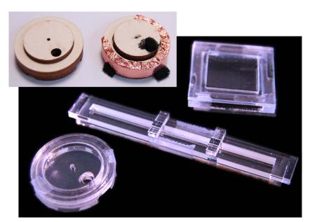
**Figure 4.3:** Cardboard + copper tape prototypes and acrylic controls.
