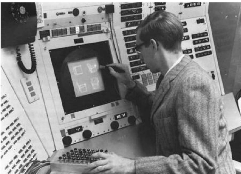
Figure 3.7: The Sketchpad system combining direct pen input on the display with physical controls for specific instruments [SUTHERLAND, 1964].
