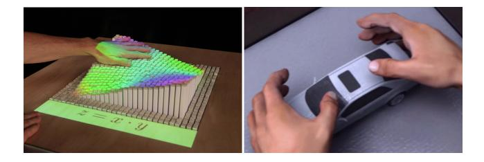
**Figure 8.8:** Technology for dynamic physical information displays: inFORM, a shape display [Follmer et al., 2013] (left), Claytronics, a concept prototype for freely programmable matter [CMU & Intel Research, 2006].
