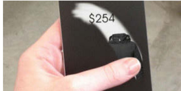
Figure 8.7: The exact value of data point can be revealed by touching a surface covered with thermochromic ink while otherwise reducing visual clutter by hiding such details.
