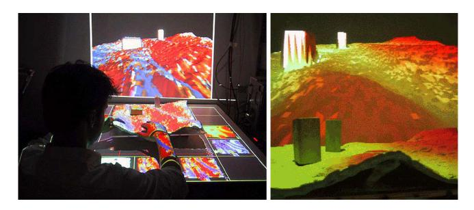
Figure 2.27: 3D tangible landscape analysis system by PIPER ET AL. [2002]
