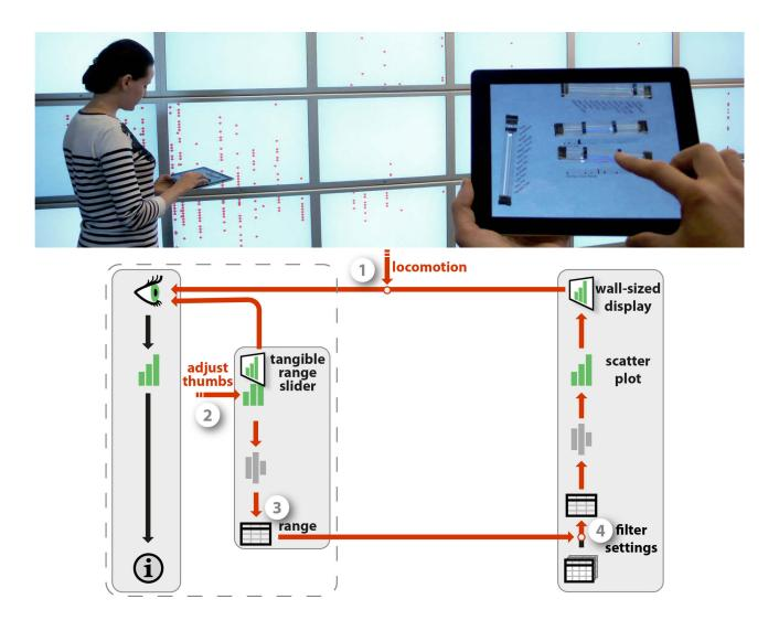
**Figure 6.21:** Tangible Remote Controllers (Chapter 4) are physical widgets attached to tablet devices that support mobile interaction with wall-size displays.
