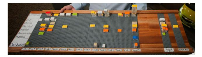
Figure 2.11: Production pipeline management used at General Motors, based on Lego bricks [WILSON, 2012].
