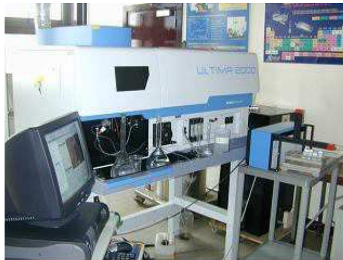
Figure II-3. Appareil ICP-AES ULTIMA 2000
