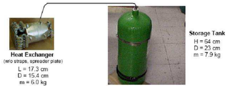
Figure 1.17: The complete system for the solid N 2 TSU[19].
