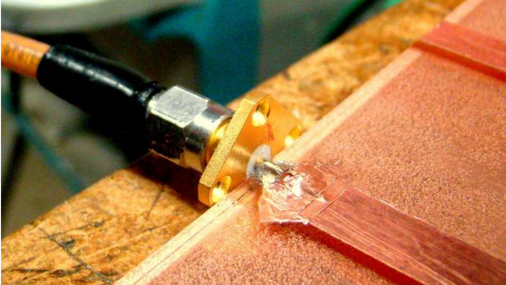
Figure 5.25 – Close-up photograph of the improved SMA connection to the micro-strip line.
