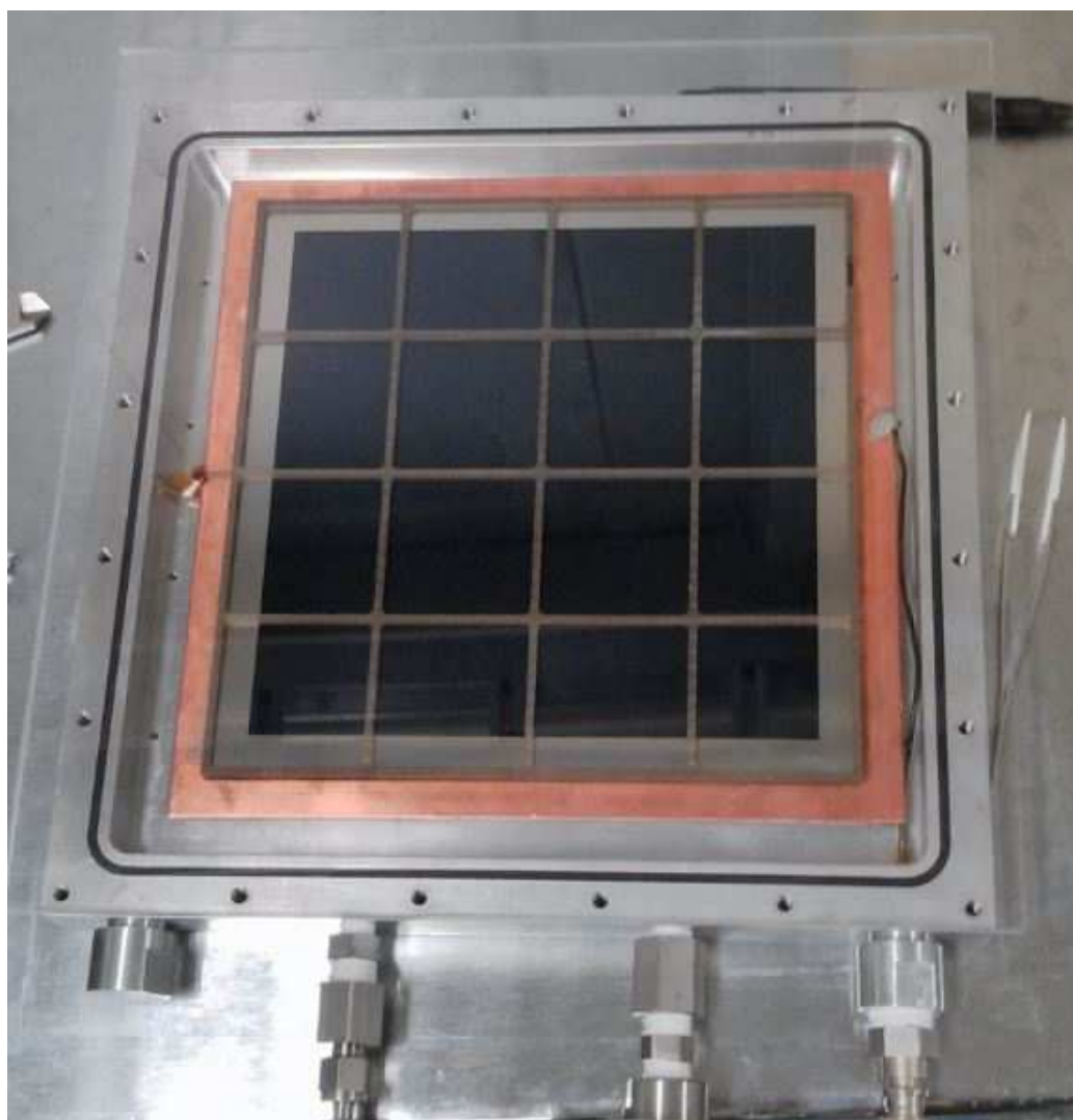
Figure 5.7 – Photograph of a test bench where no seal is required for the micro-channel plate detector. The entire stack of components is placed in a hermetic box with external vacuum applied.
