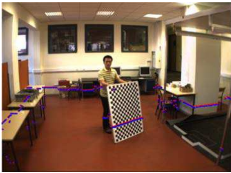
(a) Projected lidar points in the left image by two methods
