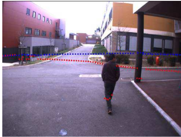
(a) Scene 1: Projection of the lidar points into the left image
