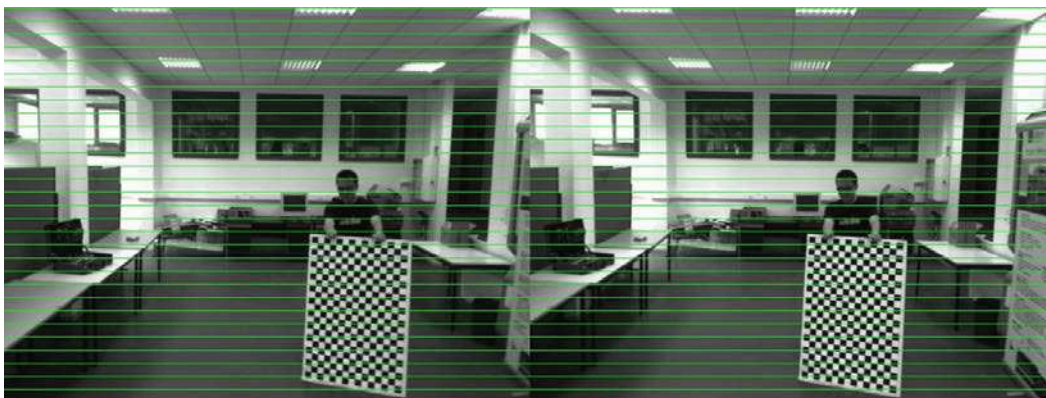
Figure 2.10: Image undistortion and stereo rectification results
