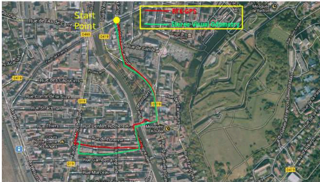
(a) Comparison between RTK-GPS and Stereo Visual Odometry
