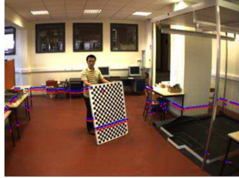
(b) Projected lidar points in the right image by two methods
