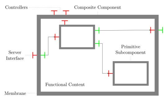
Figure 2.8 – Standard Fractal/GCM component.
