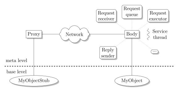
Figure 2.7 – Meta object architecture.
