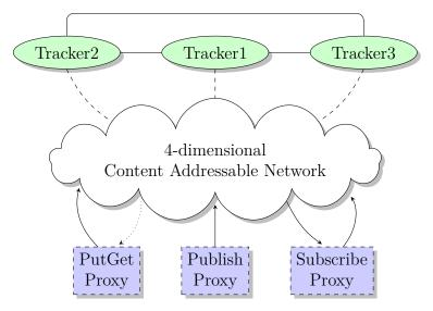
Figure 6.6 – High-level view of the EventCloud architecture.
