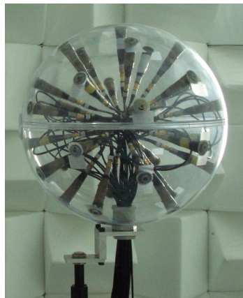
Figure 5.2: Spherical array of radius 14.5 cm with 31 microphones constructed for the validation experiments.
