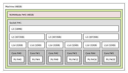
Figure 3.9: A Intel Dunnington micro-architecture Socket.
