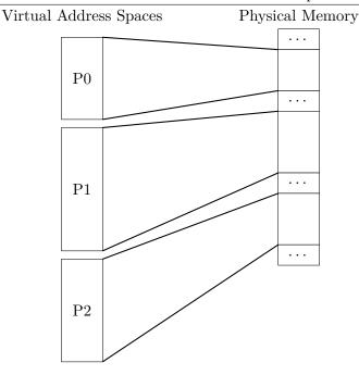
Figure 1.7: Virtual and Physical memory mapping.
