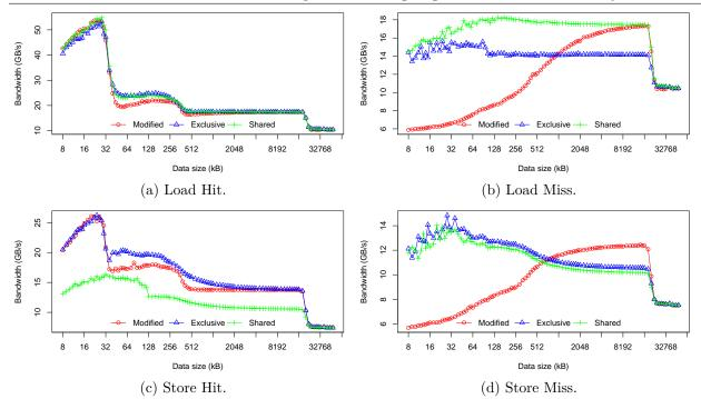
Figure 3.12: Full Benchmark Set results on Sandy-Bridge Micro-Architecture.
