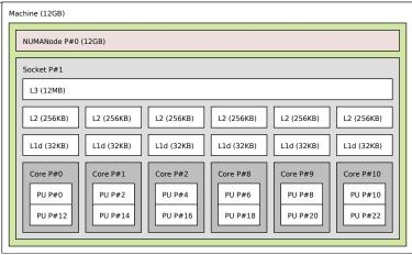
(a) A Intel Nehalem micro-architecture socket.
