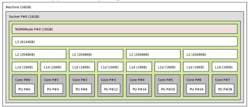
(c) A AMD Bulldozer micro-architecture socket.
