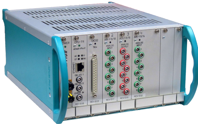
Figure 4.8.1.: Picture of the ADwin automat showing the front panel with an 18 an 14 bit analog input card an a 16 bit analog output card.
