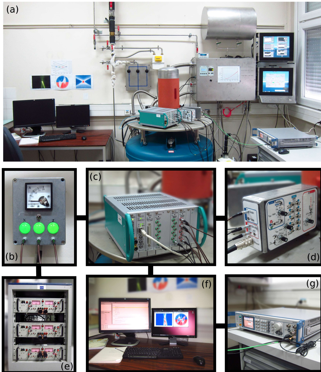
Figure 4.1.2.: (a) Picture of the experimental setup. The computer (f) controls the microwave source (g) and the ADwin real time data acquisition unit (c). The latter, in turn, operates the signal transducer (d) and the power supplies of the vector magnet, which are situated in the basement (e) via a remote terminal (b). The three LEDs in (b) indicate if the coils are operating. In case of a quench, the corresponding power supply is shut down automatically, and the LEDs will turn off. Further details of the individual parts of the experiment are explained in the text.
