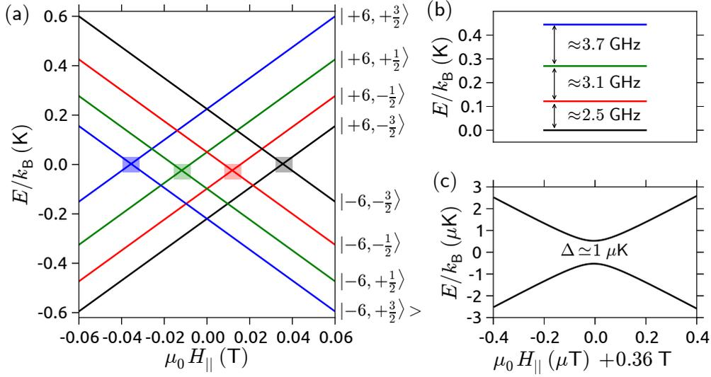
**Figure 3.7.1.:** (a) Zeeman diagram of the TbPc<sub>2</sub>. The colored rectangles indicate avoided level crossing between two states of opposite electronic spin and identical nuclear spin. (b) Energy spacing between the different nuclear spin states. (c) Magnification of the avoided level crossing between  $|6, \frac{3}{2}\rangle$  and  $|-6, \frac{3}{2}\rangle$ .
