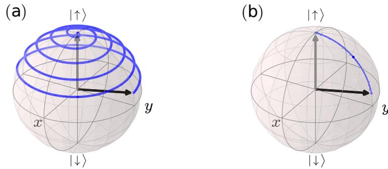
**Figure 7.1.3.:** The trajectory of a spin qubit, initialized in the  $|\uparrow\rangle$  state (grey arrow) at  $t = 0$ , was computed in the laboratory frame (a) and the rotating frame (b), while being exposed to an AC magnetic field in  $x$ -direction at resonance frequency ( $\Delta = 0$ ).
