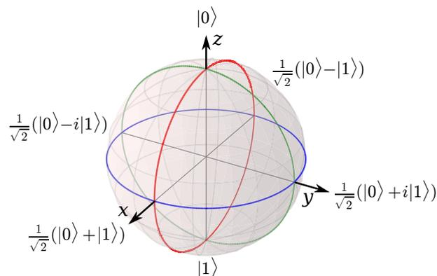
**Figure 1.2.2.:** Bloch sphere representation of a quantum bit. The two levels of a qubit  $|0\rangle$  and  $|1\rangle$  are represented by the north pole and the south pole of the sphere and any linear superposition can be visualized as a point on the surface of the sphere.
