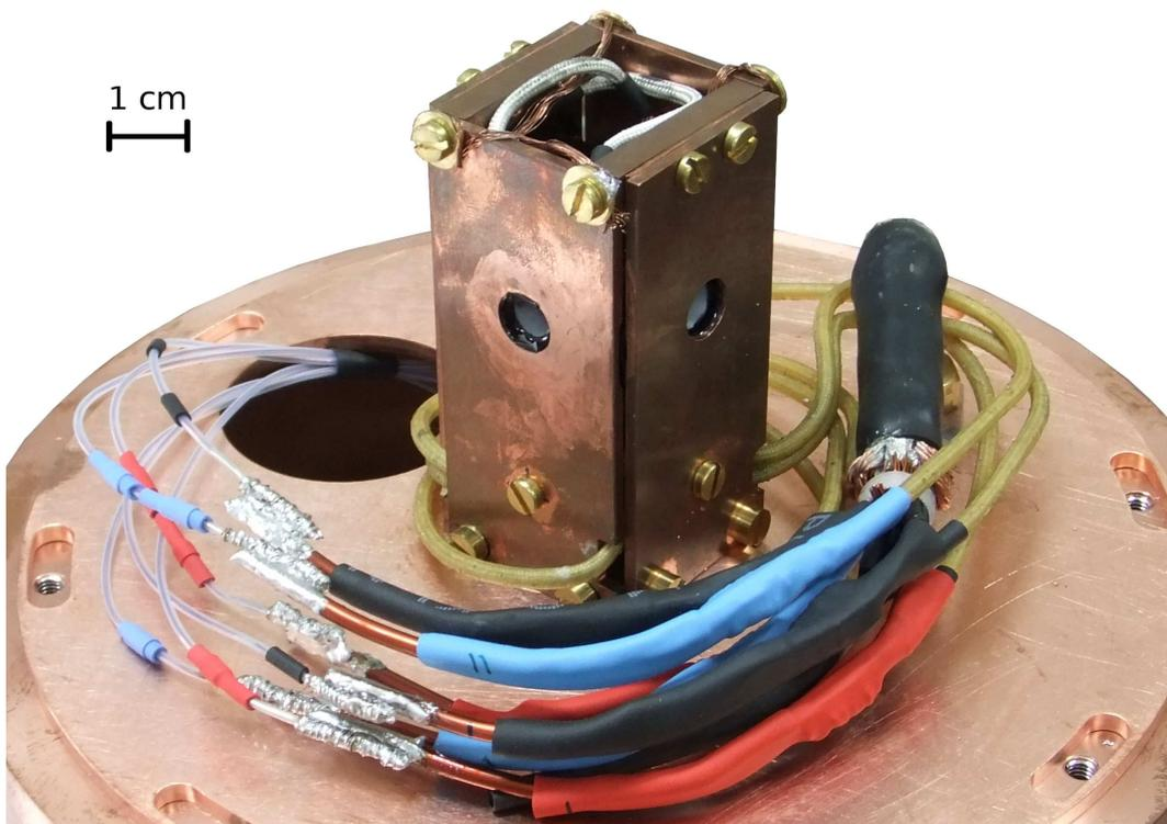
**Figure 4.3.5.:** Picture of the fully mounted vector magnet.
