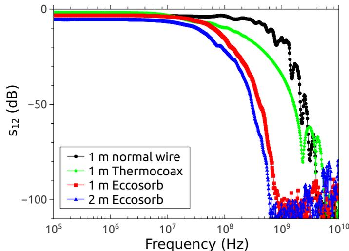
**Figure 4.6.4.:** Comparison of the attenuation of different filters. The Eccosorb filters were made out of Eccosorb-coated wires enclosed in a CuNi tube with 1.5 mm in diameter.
