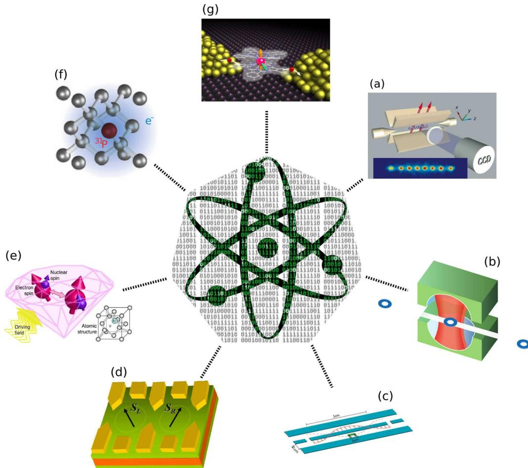
**Figure 1.2.3.:** Collection of different qubit types (a) ion traps taken from [34], (b) photons in a cavity source: Nobel Price Commite, (c) superconducting circuits taken from [35], (d) quantum dots, source: Vitaly Golovach, (e) diamond color centers taken from [36], (f)  $^{31}\text{P}$  impurities in silicon taken from [37] and (g) molecular magnets taken from [38]. Notice that selections focused on some important qubit families and is not a complete overview of all existing qubits.
