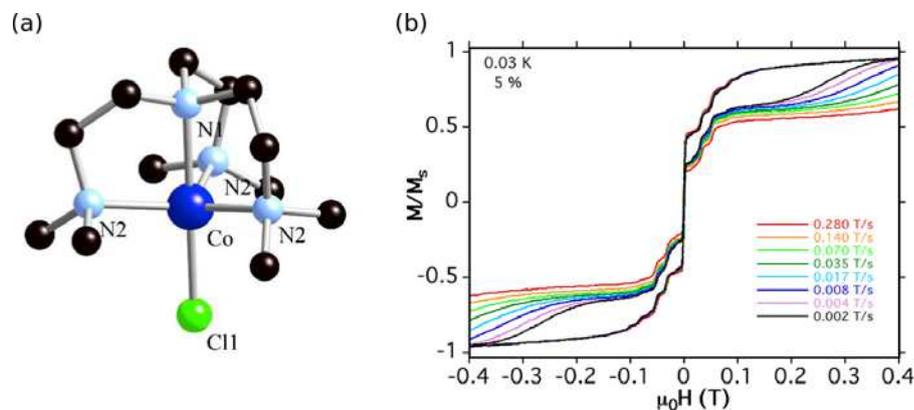
**Figure 8.0.1.:** (a) Structure of the Co(Me6tren)Cl SMM. (b) Hysteresis loop of a diluted Co(Me6tren)Cl crystal obtained with a microsquid. Steps in the hysteresis indicate the nuclear spin resolved quantum tunneling of magnetization.
