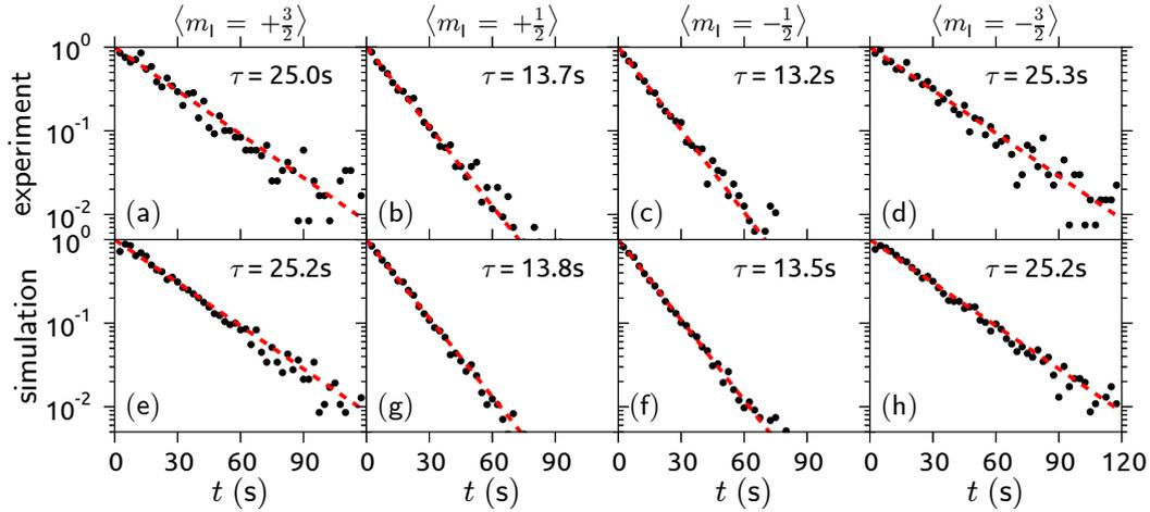
**Figure 6.4.1.:** (a)-(d) Experimental data for sample A taken from Fig. 6.2.3. (e)-(f) Computed data points using the parameters of Tab. 6.1 and the algorithm of section 6.3. The red dotted line in each subplot is a fit to an exponential function  $y = \exp(-t/T_1)$ , yielding the relaxation time  $T_1$  for each nuclear spin state.
