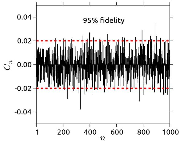
**Figure 5.7.3.:** The autocorrelation function  $C_n$  between QTM events, which were separated by  $n$  measurement (black line) and the 95% fidelity threshold indicating the randomness of the autocorrelation function (red dotted line). Since  $C_n$  is most of the time below the threshold we could reason that QTM transitions happened at random, as expected from a quantum tunneling process.
