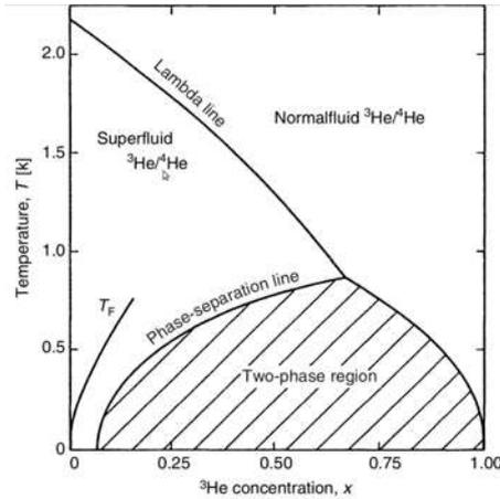
**Figure 4.2.3.:** Phase diagram of liquid  $^3\text{He}$  and  $^4\text{He}$  mixtures at saturated vapour pressure taken from [76]. Below the critical temperature of 867 mK, the mixture separates into two phases, a  $^3\text{He}$  rich and a  $^3\text{He}$  diluted phase.
