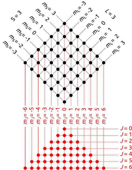
**Figure 3.5.1.:** Due to the spin-orbit coupling, the total spin  $\mathbf{S}$ , with its  $2S + 1$  states, is coupling to the total orbital momentum  $\mathbf{L}$ , with its  $2L + 1$  states, resulting in a total momentum  $\mathbf{J} = \mathbf{L} + \mathbf{S}$  with  $(2S + 1)(2L + 1)$  states.
