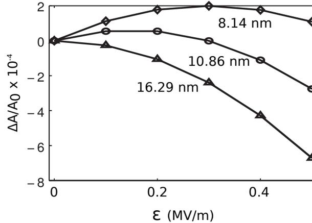
**Figure 7.1.7.:** Electric field response of the hyperfine constant at different distances between the impurity and the silicon interface. Adapted from [132].
