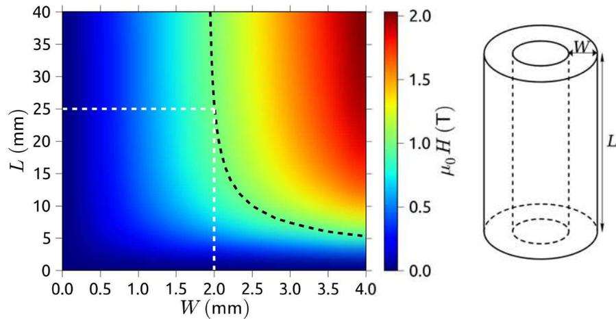
**Figure 4.3.1.:** Magnitude of the magnetic field in the center of the  $z$ -coil as a function of the coil length  $L$  and the accumulated width  $W$  of the wire layers. The black dashed line is the isofield line of 1 T. In order to reach 1 T at 10 A the minimum width needs to be 2 mm resulting in a length of 25 mm.
