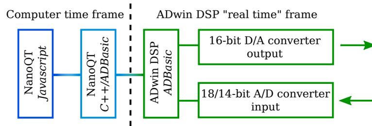
**Figure 4.8.2.:** Schematic representation of the different execution levels during the data acquisition. The user programmed Script is transcribed into different lines of C++ and ADBasic, the latter being the native language of the ADwin system. Those lines are send to the ADwin DSP who carries out the instructions at a frequency of 300 MHz.
