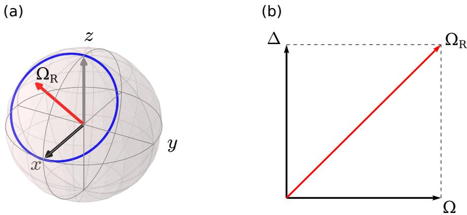
**Figure 7.1.4.:** (a) Spin precession around an effective magnetic field in the rotating frame. (b) The precession frequency  $\Omega_R$  is given by  $\Omega_R = \sqrt{\Delta^2 + \Omega^2}$ .
