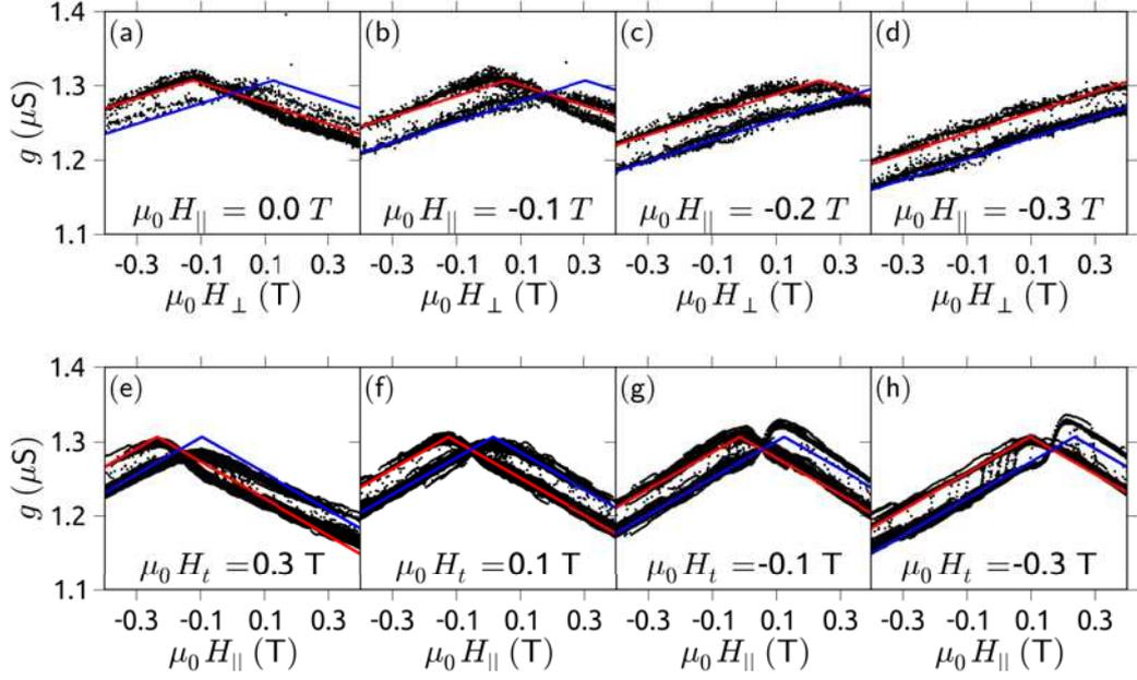
**Figure 5.5.1.:** Magneto-conductance signal of sample A as a function of the transverse field  $B_{\perp}$  at four different parallel fields  $B_{\parallel}$  (a-d) and vice versa (e-f). The red curve is an empirical fit to the spin-down conductance and the blue curve to the spin-up conductance.
