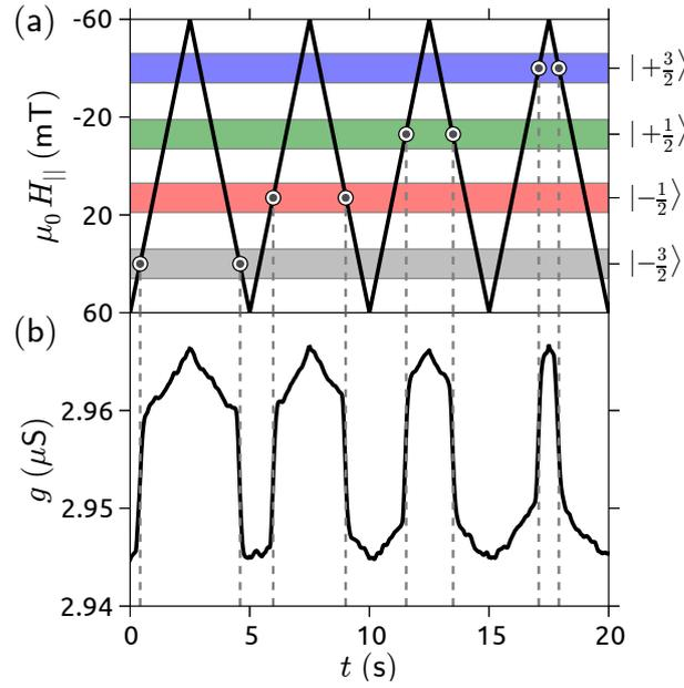
**Figure 6.2.1.:** Protocol to measure the nuclear spin trajectory. (a) The magnetic field  $B_{||}$  is swept up and down between  $\pm 60$  mT at a constant rate of 48 mT/s, corresponding to 2.5 s per sweep. (b) Each detected conductance jump can therefore be assigned to a certain nuclear spin state at a certain time  $t$ .
