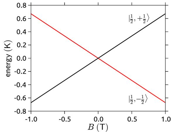
Figure 3.3.1.: Zeeman diagram of a free electron.
