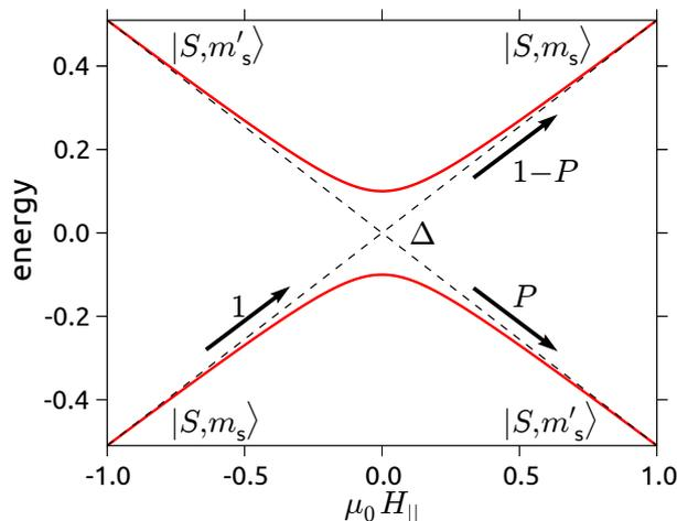
**Figure 3.8.2.:** Avoided level crossing between the two states  $|S, m_s\rangle$  and  $|S, m_s'\rangle$ , which leads to the quantum tunneling of magnetization. While sweeping the parallel field over the anticrossing the probability  $P$  to tunnel from one state into the other is given by the Landau-Zener formula (Eq. 3.8.1).
