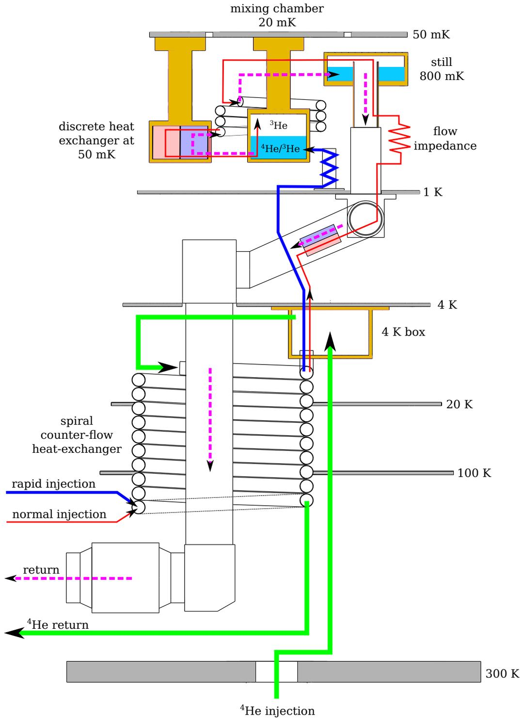
**Figure 4.2.1.:** Schematic of an inverted dilution refrigerator. The secondary cooling circuit (green) is precooling the primary circuit consisting of the normal injection (red) and rapid injection (blue). The latter is only used during the cool down from room temperature. During the steady state operation,  ${}^3\text{He}$  is injected via the normal injection into the  ${}^3\text{He}$  rich phase of mixing chamber and extracted from the diluted phase (violet).
