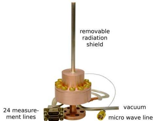
**Figure 4.5.1.:** Radiation shield with a independent vacuum, a feed through of 24 measurement lines and one microwave line.
