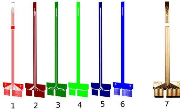
**Figure 4.5.2.:** (1-6) Layout of the chip carrier consisting of six independent layers. The top three layers contain the 24 DC strip lines and three bottom layers  $50\ \Omega$  matched waveguide. (7) Picture of the sample holder.
