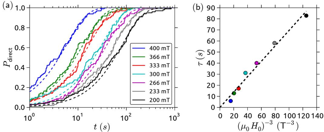
**Figure 5.6.1.:** (a) The solid lines represent the relaxation probability  $P_{\text{direct}}$  as a function of the waiting time  $t$  at different magnetic fields  $H_0$ , which are indicated in the legend. The dashed lines are a fit to  $P_{\text{direct}} = 1 - \exp(t/\tau)$ . (b) Characteristic relaxation time  $\tau$  extracted from the fits of (a) as a function of  $H_0$ .
