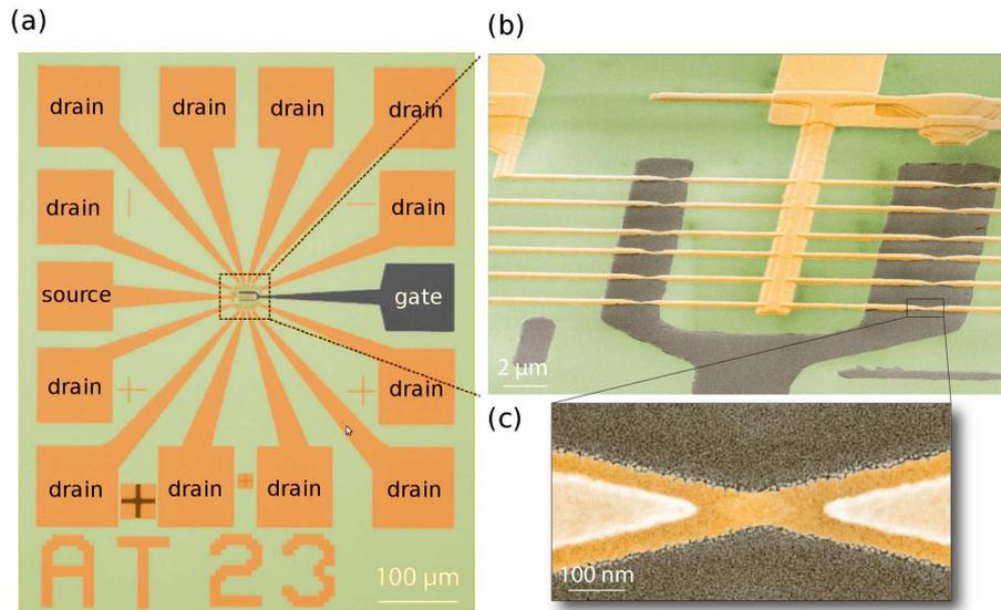
**Figure 4.9.1.:** (a) Layout of an array of 12 transistors sharing a common source and gate terminal. (b) Scanning electron microscope image showing the back gate (grey) as well as the common source and the different drain terminals. (c) Zoom showing the nanowire obtained by shadow mask evaporation.
