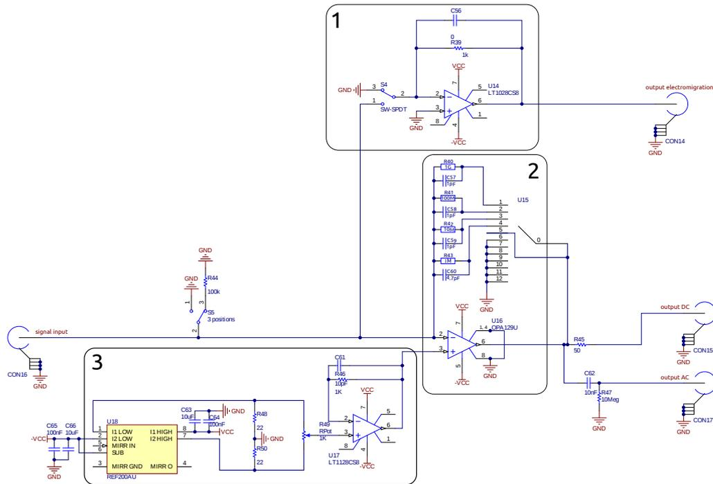
**Figure 4.7.1.:** Circuit diagram of the IV converter. Box (I) contains the fast current voltage converter with a bandwidth of 1 MHz and an amplification of  $10^3$ . This IV converter is used for the electromigration only. Box (2) shows the ultra low noise IV converter with 4 selectable gains used for the electrical transport measurements. The offset of the IV converter in (2) is adjusted by the circuit embedded in (3).
