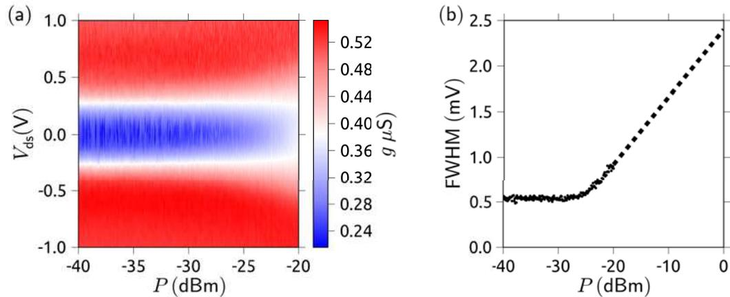
**Figure 7.3.2.:** (a) Conductance through the read-out dot as a function of the source-drain voltage  $V_{\text{ds}}$  and the applied microwave power  $P$ . (b) Evolution of the full width half maximum (FWHM) of the dip in (a) as a function of the microwave power  $P$ .
