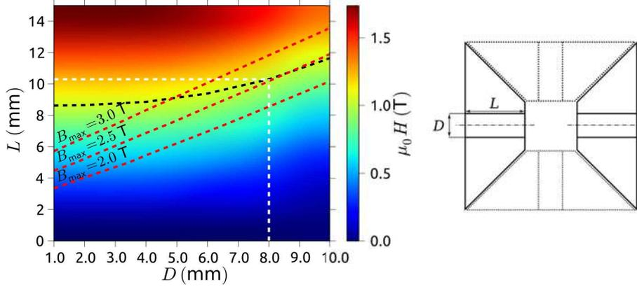
**Figure 4.3.3.:** Magnitude of the magnetic field in the center of the two conically shaped split coils as a function of the inner diameter  $D$  and the thickness  $L$ . The black dashed line is the isofield line of 1 T. The red line correspond to the maximum field at the inner wall of the coils. In order to reduce that maximum field, we set the dimensions to  $D = 8$  mm and  $L = 10$  mm.
