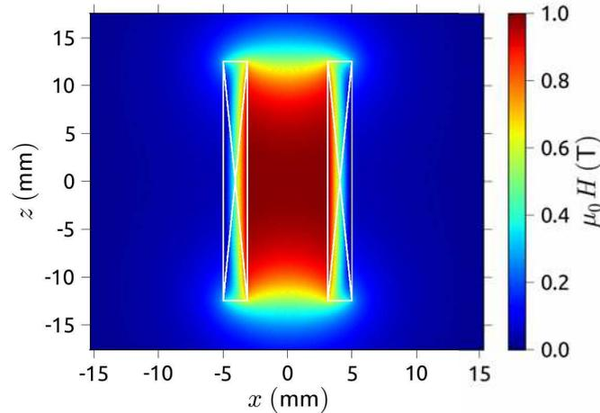
**Figure 4.3.2.:** Cross section of spacial magnetic field distribution of the  $z$ -coil at  $y = 0$ . A homogeneous field of about 1 T can be found in a radius of 3 mm around the center of the coil. Note the rotation symmetry of the field distribution around the  $z$ -axis.
