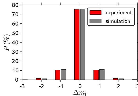
**Figure 6.4.5.:** Histogram of all transitions observed in the experiment (red) and simulation (grey). Transitions with  $\Delta m_I \neq \pm 1$  correspond to multiple transitions of  $\Delta m_I = \pm 1$ , which were not resolved due to the finite time resolution.
