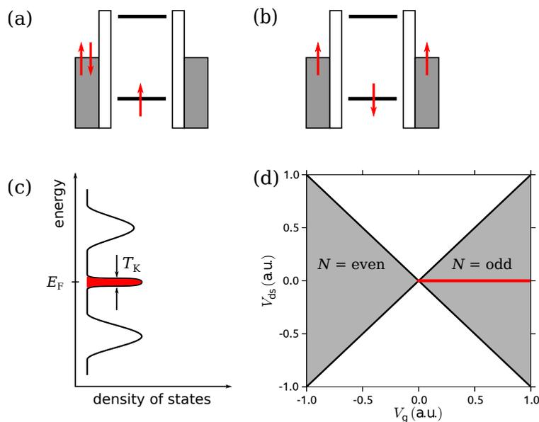
**Figure 2.4.1.:** Kondo transport mechanism with the initial state (a) and the final state (b). Note that the spin of the quantum dot flipped during the process. (c) The Kondo effect creates a peak in the density of states, whose width is given by the Kondo temperature. (d) Experimentally, the Kondo effect is observed as a conductance ridge or Kondo ridge (red line) inside the Coulomb blockade region of the stability diagram
