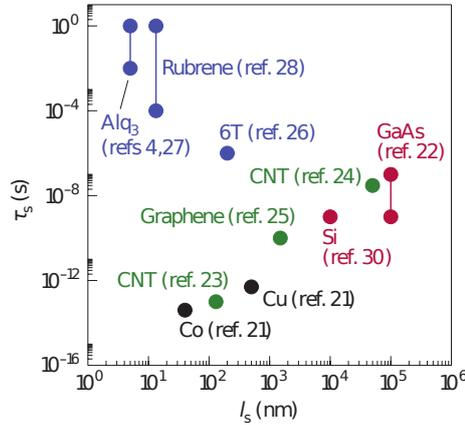
**Figure 1.1.1.:** Spin-relaxation time  $\tau_s$  versus spin-diffusion length  $l_s$ . Organic semiconductors are situated in the upper left corner corresponding to long spin-lifetimes but short diffusion lengths. The figure was taken from [6], and the used references correspond to the ones from [6].
