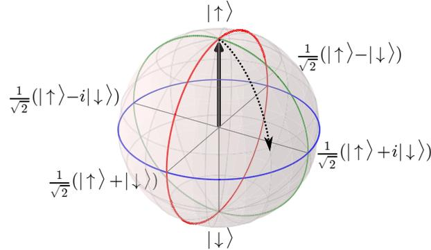
**Figure 7.1.1.:** Bloch sphere representation of a two level spin qubit system. The north and south pole of the sphere correspond to the two eigenstates  $|\uparrow\rangle$  and  $|\downarrow\rangle$ , whereas the qubit state is indicated as a vector, which can be at any point on the surface. A coherent manipulation of the qubit is shown as a rotation of the vector on the sphere. Note that the trajectory of the rotation was chosen arbitrary and has no further meaning.
