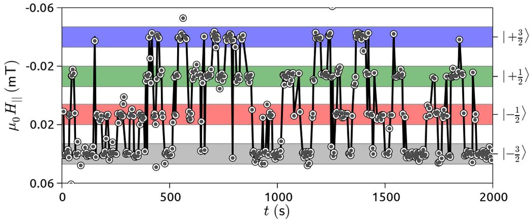
**Figure 6.2.2.:** First 2000 s of the nuclear spin trajectory measured using sample A. The grey dots illustrate the recorded conductance jump. If the jump was found inside a window of  $\pm 7$  mT (colored stripes) around one of four peaks of Fig. 6.1.1(d) it was assigned to the corresponding nuclear spin state, otherwise the measurement was rejected. Using this data analysis results in the single nuclear spin trajectory, shown as a black line.
