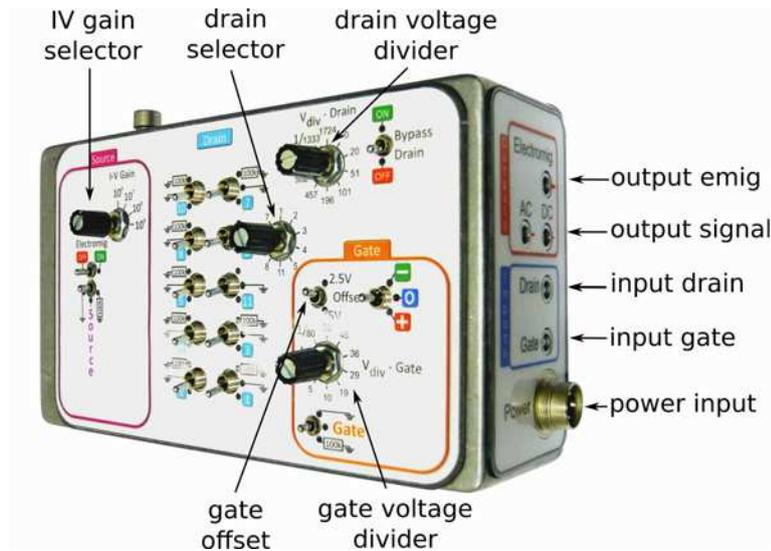
**Figure 4.7.3.:** Picture of the signal transducer.
