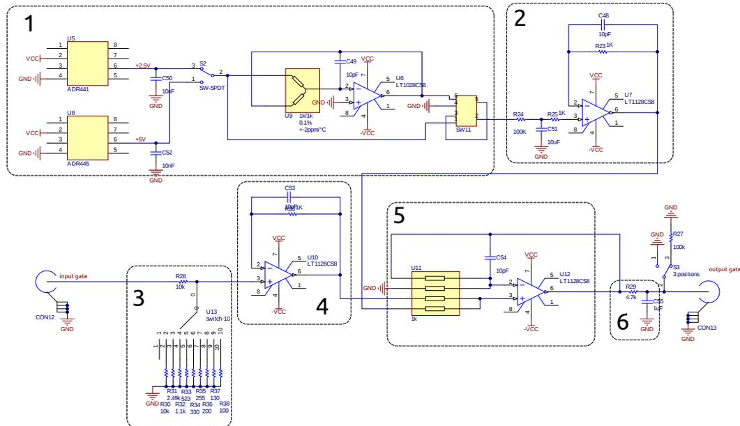
**Figure 4.7.2.:** Schematic of the gate circuit. Circuit diagram of the gate circuit. The input gate voltage is divided using the circuit in box 3. Subsequently an optional offset of 0 V,  $\pm 2.5$  V or  $\pm 5$  V is generated using the circuit in box 1 and added to the divided signal using the summing amplifier in box 5. The circuit in 2 and 4 are used to match the output impedances of 3 and 1 to 5.
