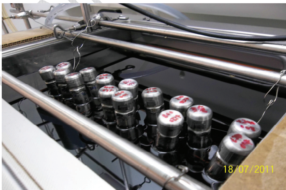
Figure II-7: Stainless steel tubes in hot oil bath for dilute acid hydrolysis
