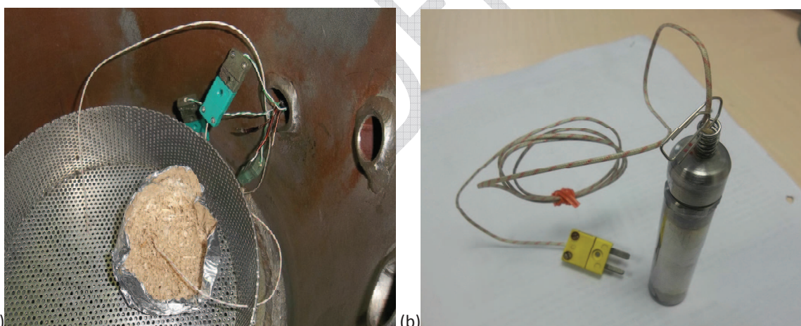
Figure III-48: (a) Two thermocouple probe with one attached to the product and the other one exposed to reactor environment (b) Stainless steel reactor used for non-isothermal study.
