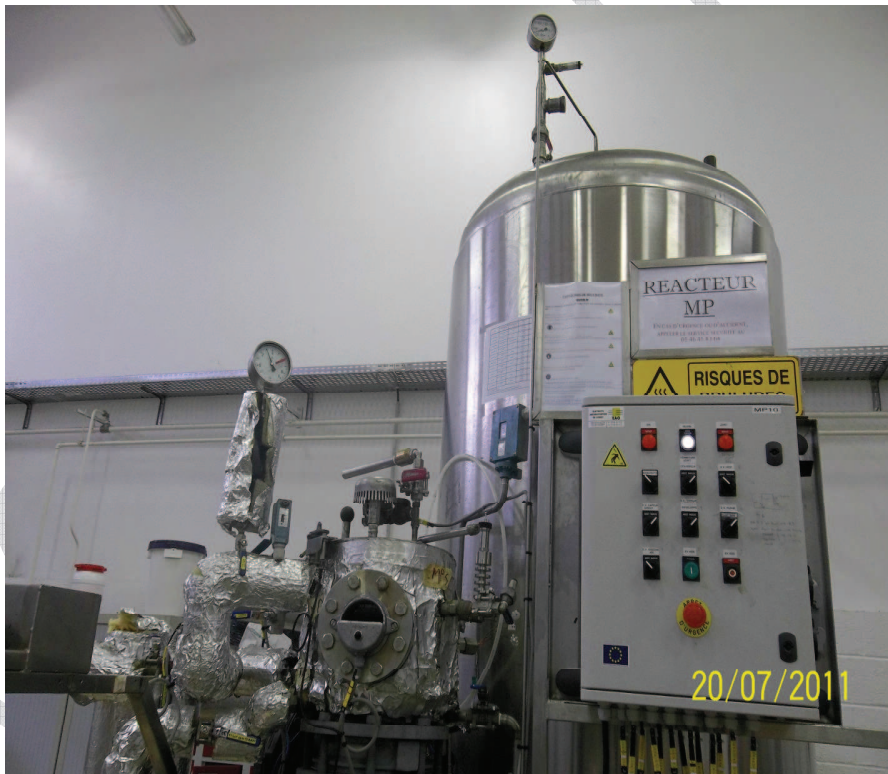
Figure I-17: DIC reactor used in this work was MP system (with medium steam pressure)
