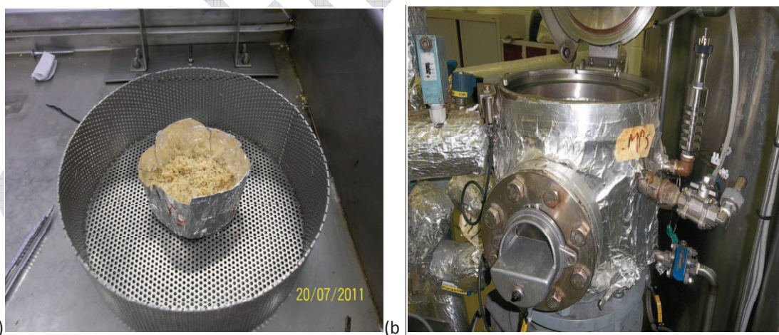
Figure II-6: (a) Sample holder and sample container used in this study (b) DIC reactor chamber for thermal pretreatment
