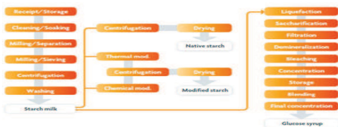
Figure I-2: Processing chart for glucose production from starch obtained from cereals. [Adapted from - http://www.tereos.com/en-gb/activites/filieres/cereales.html ]
