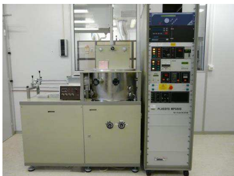
Sputtering machine (for Al & Pt)
