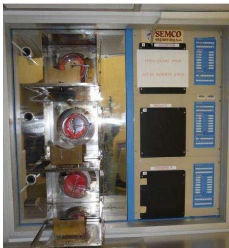
Oxidation and annealing ovens
