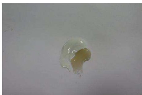
55b: two-component gastight epoxy resin, before (left) and after (right) mixing
