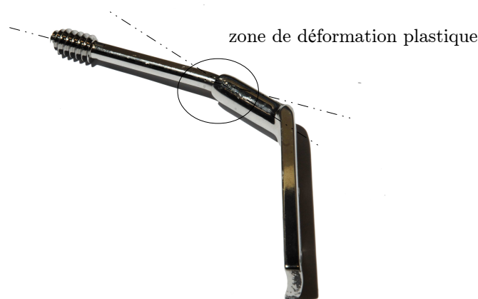
Figure 4.35 – Plastification de la vis céphalique de la plaque DHS.
