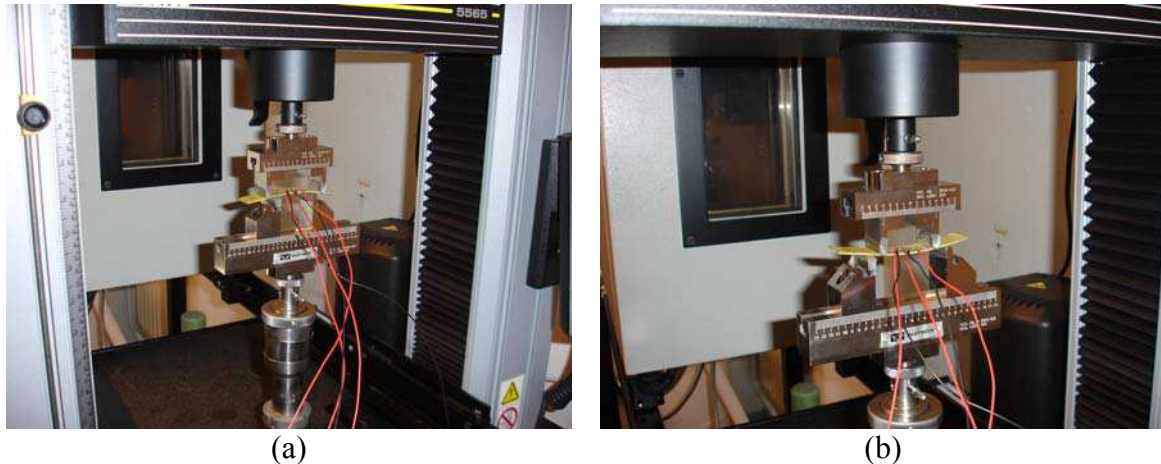
Figure 5.34 Substrat FR-4 sous flexion (a) Traction - Compression, (b) Compression - Traction
