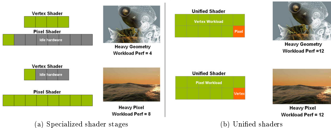
Figure 2.8: Unified computing shader units allow to achieve better performances in any application case. Courtesy of NVIDIA.
