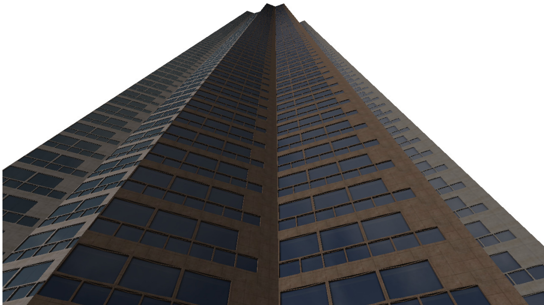
Figure 7.12: The skyscrapers comprise up to 209 floors, generated in 21ms and rendered at a minimum of 38.4fps using our massive management system within the GPU shape grammars pipeline.
