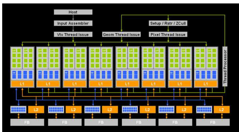
Figure 2.7: G80 architecture based on Streaming Multiprocessors. Courtesy of NVIDIA.
