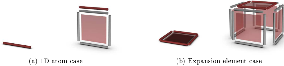
Figure 4.7: Starting from a single 1D atom (a), our segment-based formulation generates an expansion element (i.e., a 2D atom and a set of contour 1D atoms) and the initial 1D atom is translated. We may also start from such an expansion element (b): each contour 1D atom is segment-based expanded as in (a) and the 2D atom is translated.
