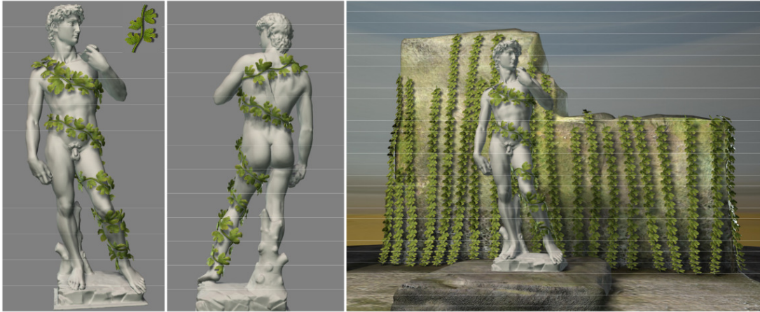
Figure 3.12: A 3D sample of an ivy's stem and leaves is applied on the David mesh. With a vector field, the artist can design the final, complex mesh by guiding the mesh quilting algorithm. Here, the ivy is made to wrap around the leg and climb to the torso. Image from [ZHW + 06].
