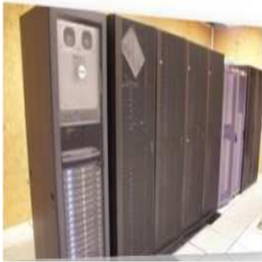
Figure 3.6: The Nef Torque cluster, at INRIA Sophia-Antipolis research center. A cluster with 37 nodes and 876 processors.
