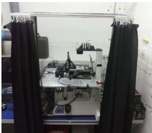
Figure 5.11: The MEA cage. A Faraday cage to avoid the electrostatic noise.
