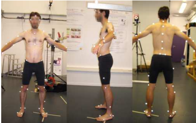
Figure 3.3: Calibration procedure for positioning markers regarding the subject's body. The photographs are taken in respectively face, left profile and back directions.
