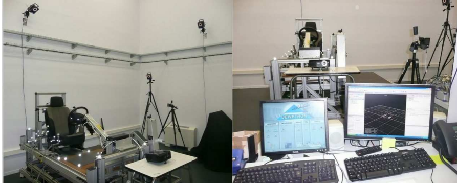
Figure 3.1: Mocap rooms with experimental devices - Vicon ® cameras and PC (Source: website of LBMC).
