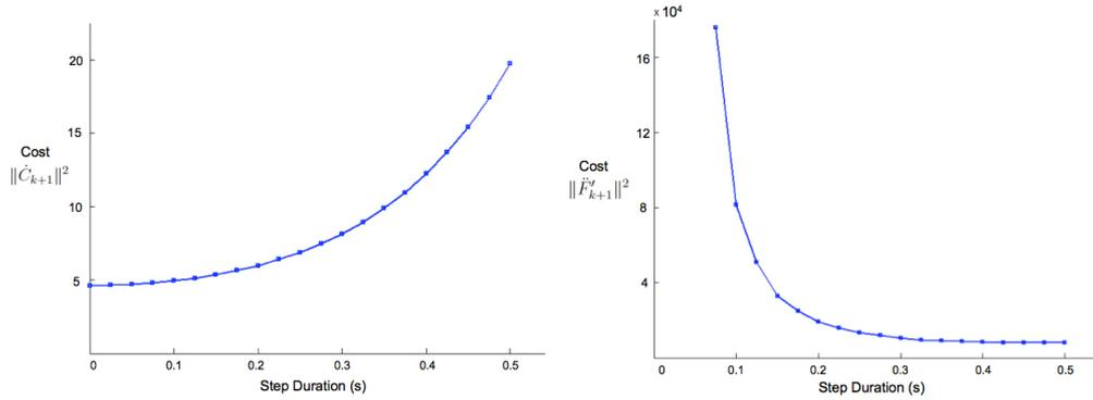
**Figure 4.7:** The CoM velocity cost (left) and swing foot acceleration cost (right) against varying step durations and for step lengths plotted in Figure 4.6. Note that both the costs show completely opposite trend against step duration
