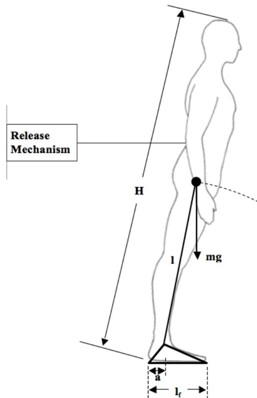
**Figure 3.11:** The representation of the human body used for the so-called *mechanical* model. It consists of a simple inverted pendulum + foot model, where the CoM follows a circular arc around the ankle joint.
