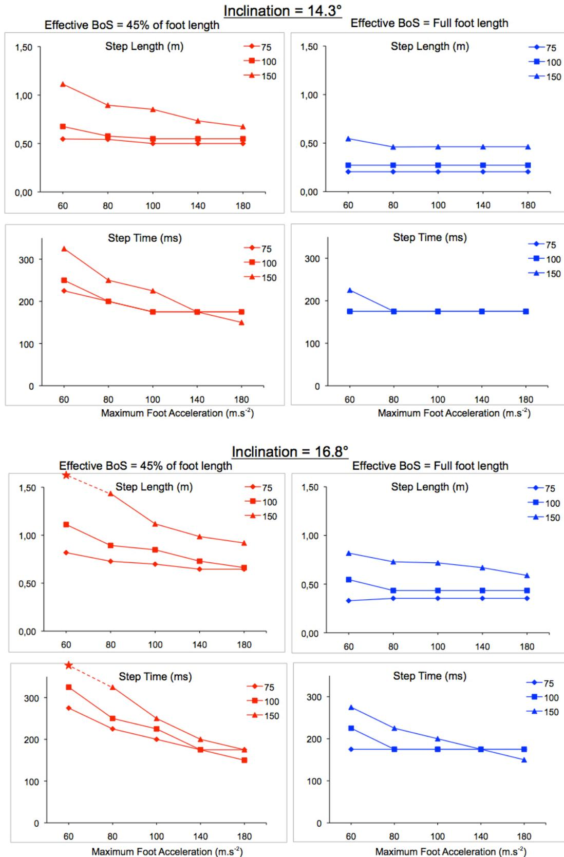
**Figure 5.14:** Optimized step lengths and timings against forward inclinations scenario for elderly from Hsiao-Weckslar and Robinovitch (2007) against maximum foot acceleration values (varied along x-axis) for 3 different reaction time values (75, 100 and 150 ms) and 2 different effective BoS lengths: (left red plots for reduced BoS vs. right blue plots for full BoS). Starred value (★) represents a fall.
