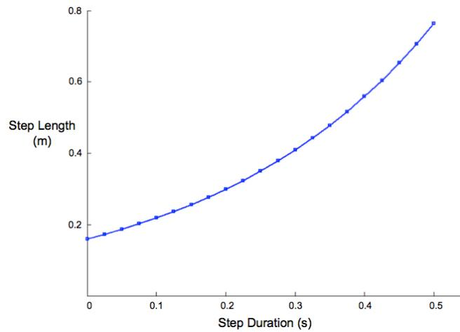
**Figure 4.6:** Single recovery step lengths for a given perturbation as function of step durations
