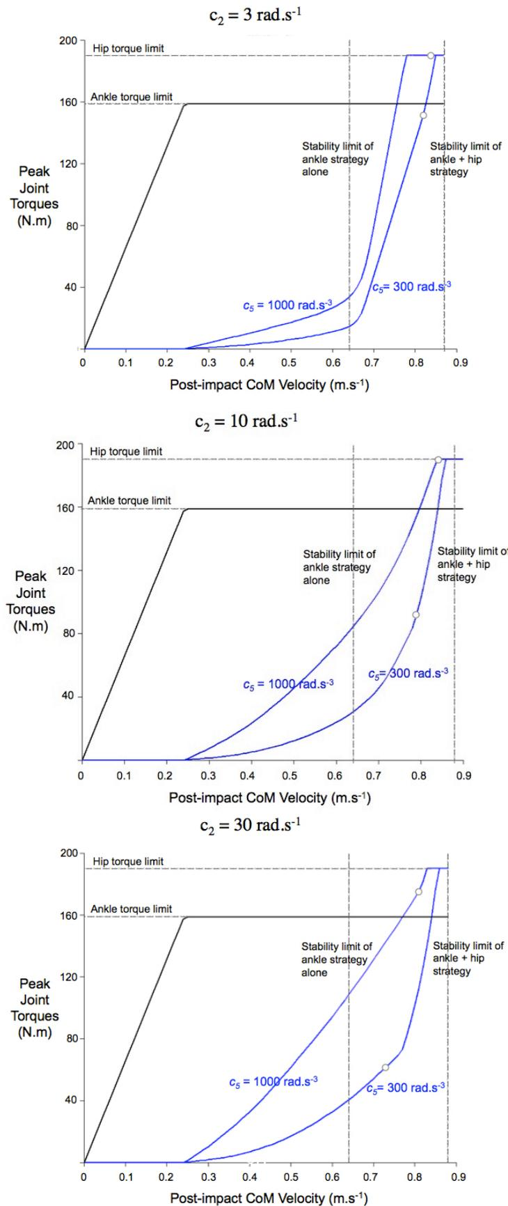
**Figure 4.11:** The relative level of use of ankle and hip strategies. Peak ankle (black) and hip (blue) torques are plotted against varying perturbations. White dot indicates the point where upper-body angle limit of  $90^\circ$  is reached
