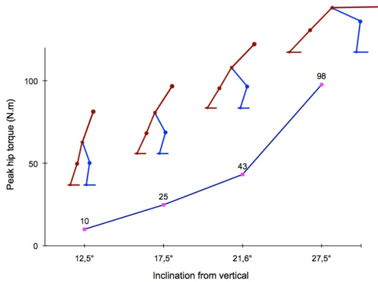
**Figure 4.17:** The peak hip torque values achieved during the 4 recovery scenarios from Hsiao-Wecksler and Robinovitch (2007) and corresponding final recovery postures of the mechanical model. Note that the peak hip torque and upper-body rotation angle are positively scaled with the perturbation level.
