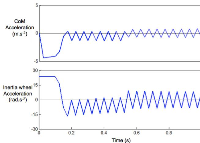
**Figure 4.4:** Time profiles of CoM and inertia wheel accelerations following a given disturbance obtained by minimizing cost function (4.23). Note the resulting fluctuations due to the absence of their third derivative penalization
