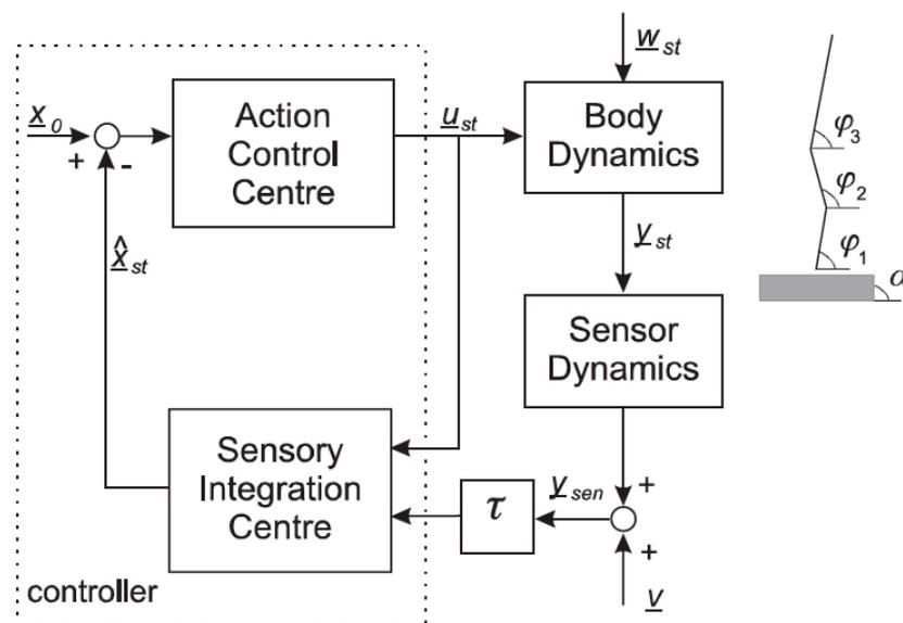
**Figure 2.7:** Flow diagram of the human stance control model proposed by van der Kooij et al. (1999). The unknown disturbances  $w_{st}$  are successfully offset by the muscle actions  $u_{st}$ . In addition to sensory input, the sensory control center also inputs muscle actions for best estimate of the body sway
