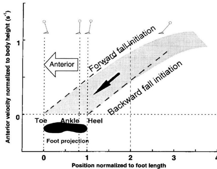
**Figure 2.5:** The stability of ankle strategy calculated in Pai and Patton (1997) (shaded region) and approximated by Hof et al. (2005) (dotted line) using a simple inverted pendulum model. (Figure taken from Hof et al. (2005))
