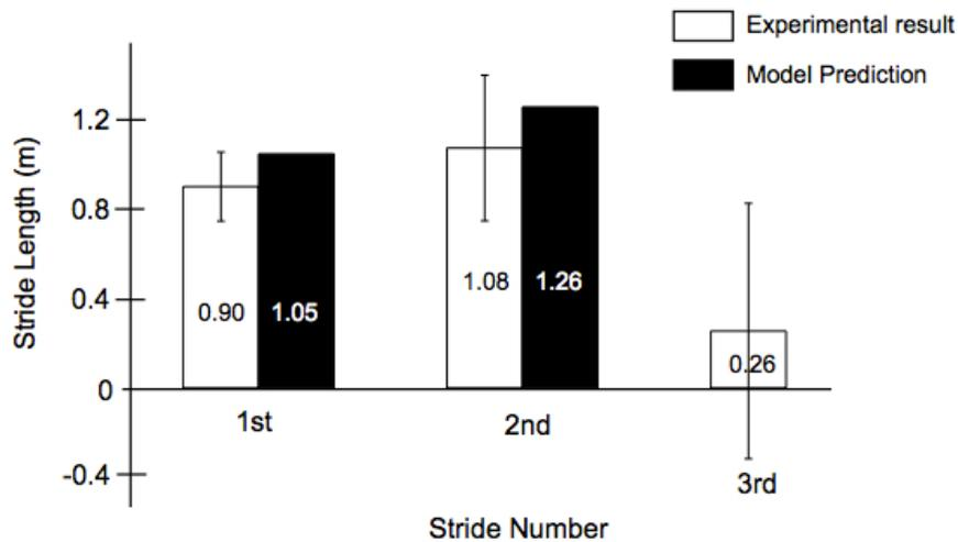
**Figure 3.14:** Stride length for multiple step recovery scenario from Cyr and Smeesters (2009a). Experimental (white bars, averaged across subjects  $\pm$  one standard deviation) versus simulated (black bars) results.
