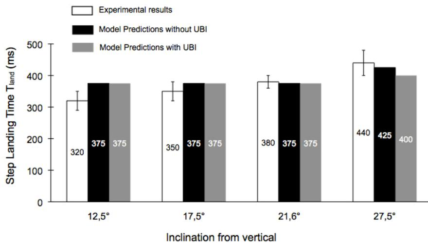
**Figure 4.21:** The predicted step landing times  $T_{land}$  for the 4 perturbation scenarios of Hsiao-Wecksler and Robinovitch (2007), with and without UBI considerations compared against experimental values (white bars)
