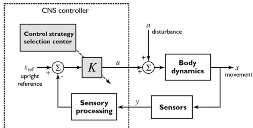
**Figure 2.6:** A linear feedback control model, where  $K$  is a matrix of feedback gains producing joint torque commands  $u$  as a function of body movement  $x$  (Park et al., 2004).
