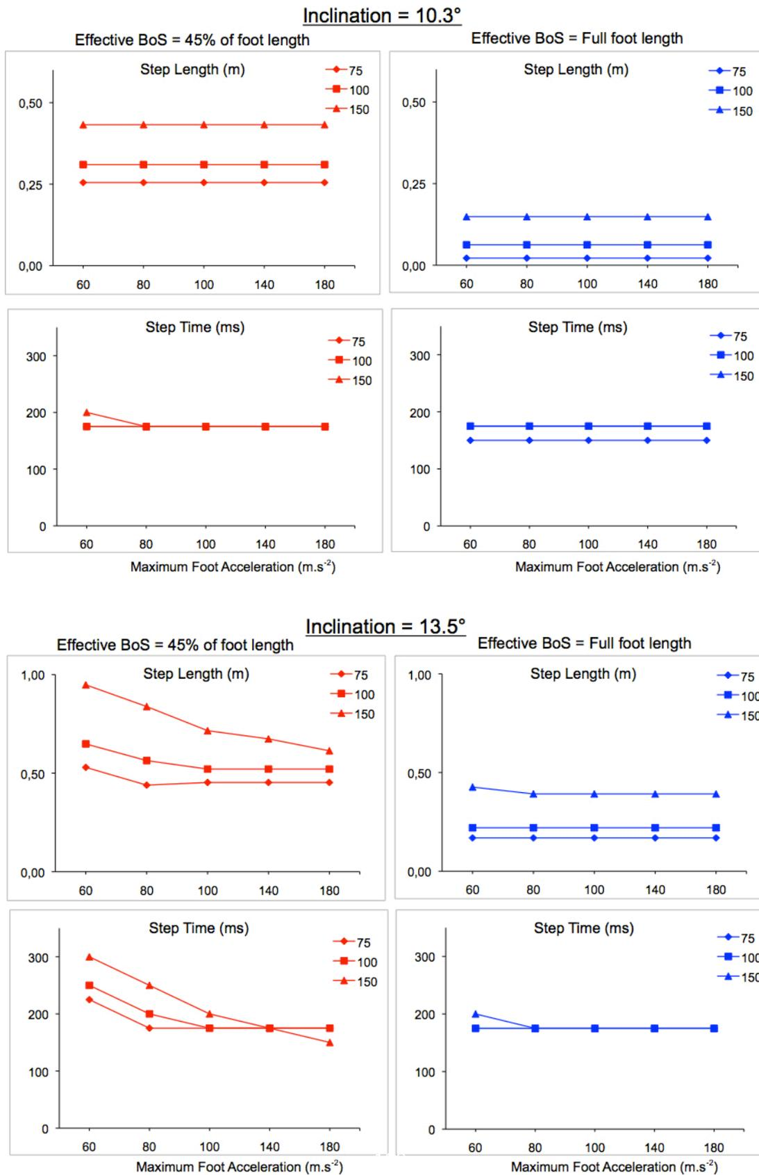
**Figure 5.13:** Optimized step lengths and timings against forward inclinations scenario for elderly from Hsiao-Wecksler and Robinovitch (2007) against maximum foot acceleration values (varied along x-axis) for 3 different reaction time values (75, 100 and 150 ms) and 2 different effective BoS lengths: (left red plots for reduced BoS vs. right blue plots for full BoS).
