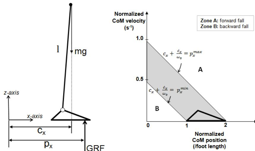
**Figure 2.8:** Left: The simple Inverted Pendulum (IP) + Foot model assumes point mass concentrated at CoM. The ground reaction force (GRF) acts at the CoP which is constrained to remain within the foot. Right: The limits of the dynamic stability region (grey area) for standing balance. Any state that lies within this region would successfully terminate its motion over the BoS (foot).
