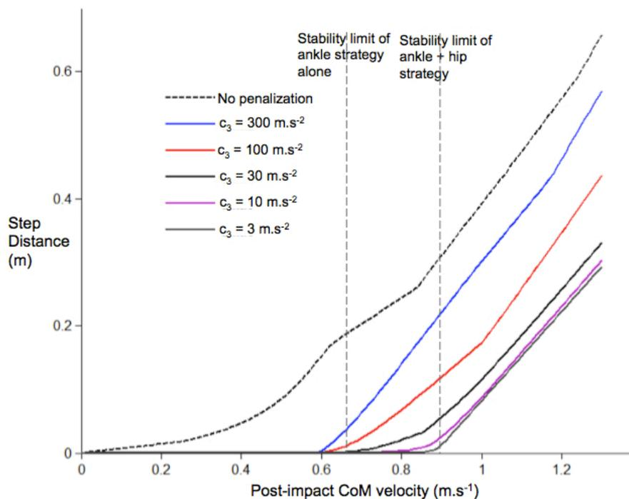
**Figure 4.14:** Step length when reacting to varying post-impact CoM velocities for different penalization coefficients  $c_3$ , or for no penalization at all of the swing foot acceleration  $\ddot{F}'_{k+1}$
