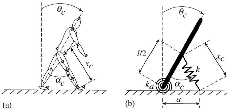
**Figure 3.6:** The stepping model of Hsiao and Robinovitch (1999) with torsional and linear springs in stance and stepping feet respectively
