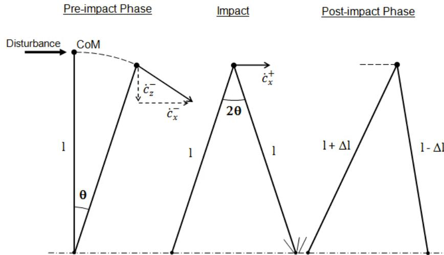
**Figure 3.2:** The stepping model proposed by Hofmann (2006) and extended by Stephens (2007). The system behaves like a simple inverted pendulum until impact with constant leg length  $l$ . After impact, the leg lengths are adjusted to move CoM at a constant height from ground.
