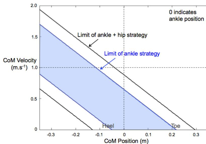
**Figure 4.3:** The fixed-support stability region in CoM state space with our MPC controller (4.23) using anthropometric parameters. Zero indicates the position of ankle in sagittal plane. It is evident that the disposition of upper-body allows recovering from much larger disturbances than with ankle strategy alone without stepping
