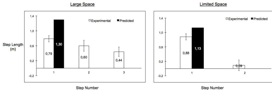
**Figure 5.5:** The simulation of two balance recovery tasks (large space vs. limited space) using the same controller parameters (c.f. Table 5.2.) The predicted stepping behavior is closer to the limited space experimental scenario (right) than with the large space.
