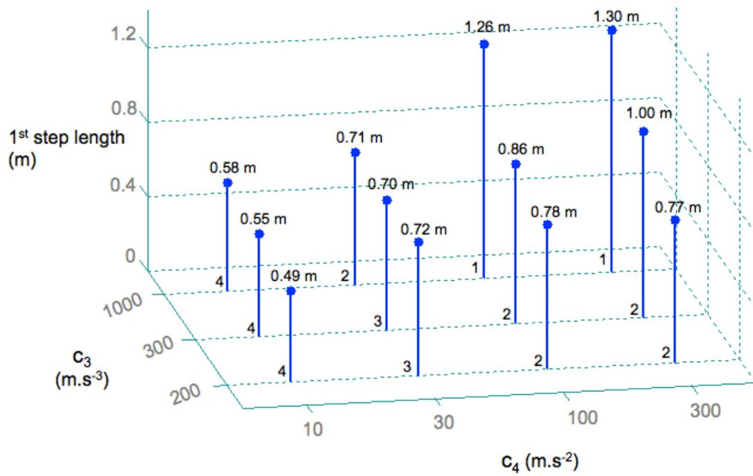
**Figure 5.6:** The lengths of predicted first step against varying values of control weights  $c_3$  and  $c_4$ , which penalize the CoM jerk and swing foot acceleration terms respectively. The number at the bottom of each plot represent the total number of predicted forward steps. It can be seen that the smaller control weight values (implying stronger penalization of corresponding cost function terms) result in shorter step lengths and more steps.
