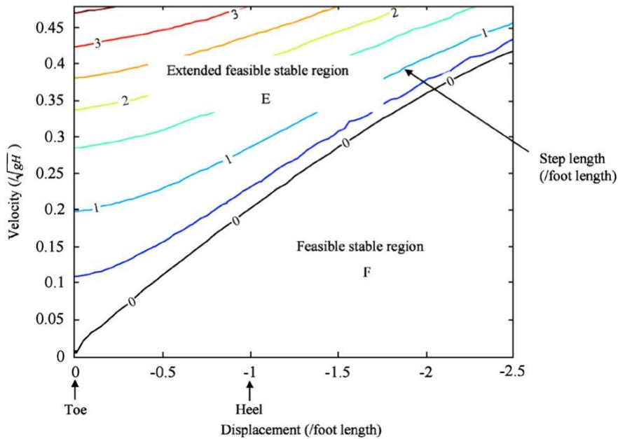
**Figure 3.5:** Minimal step length (normalized with the length of foot) needed for balance recovery of various initial displacements (normalized by the length of foot) and velocities (normalized by the  $\sqrt{gH}$ , where H is height of body and g is the acceleration due to gravity) of COM by (Wu et al., 2007)
