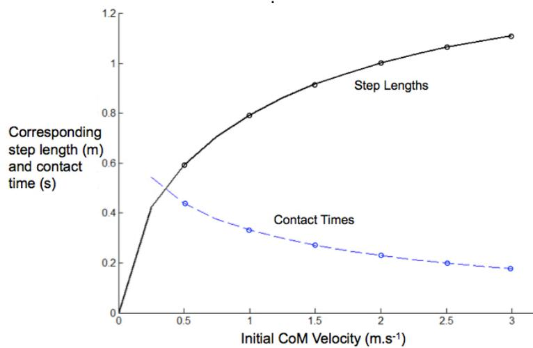
**Figure 3.4:** The optimum step lengths (black) and corresponding contact times (blue) for varying levels of initial velocity disturbances.
