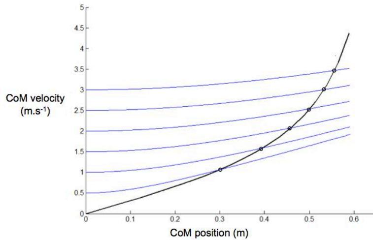
**Figure 3.3:** The trajectories under inverted pendulum model assumption from different levels of initial disturbance (blue curves) intersect the optimal step curve (black) at optimal step distance shown in Figure 3.4
