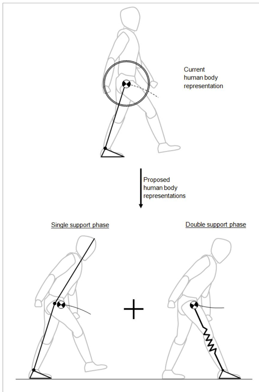
**Figure 6.1:** The current human-body representation (top) can be replaced by more realistic models such as a double-inverted pendulum (DIP) model during the single-support phase and a spring model during the double-support phase.
