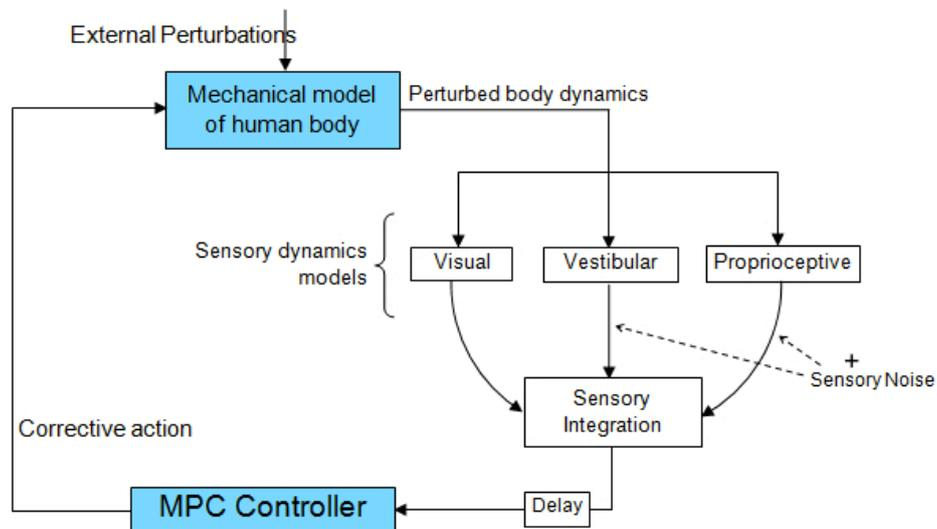
**Figure 6.2:** A possible integration of human sensory systems in the BR tool would involve a separate sensor dynamic model of each sensory modality ((e.g. Borah et al., 1988)) and a sensory integration center.
