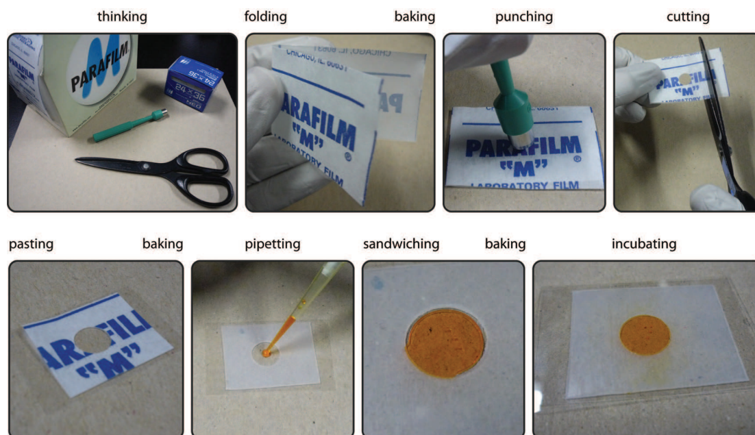
Figure 6.9: Making of Paraframe chambers.
