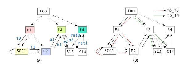
Figure 5.8: (A) SSA-PDG after typed fusion. (B) Data Flow Program Dependence Graph.
