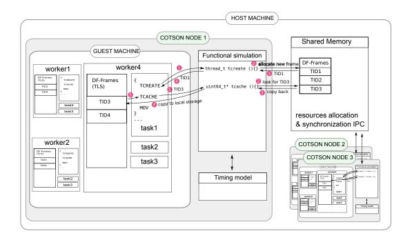
Figure 7.2: Multiple nodes simulation on COTSon.
