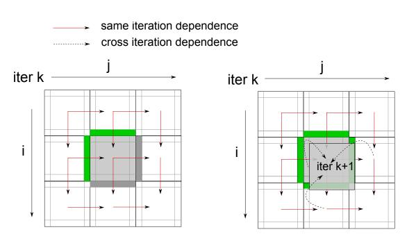
Figure 7.11: Dependence of gauss seidel: A. same iteration dependences (left) B. cross iteration dependences (right)
