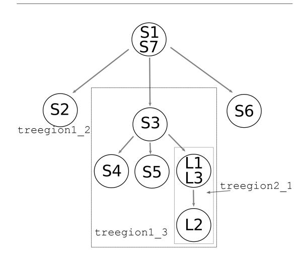
Figure 3.8: Control dependence graph of Figure 3.3. Express the definition of treegion.
