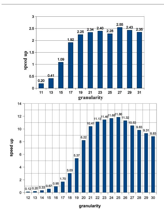
Figure 5.15: Computing the  $42^{\text{th}}$  Fibonacci number on 4 cores (above) and 24 cores (below).
