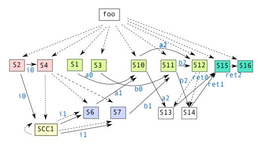
Figure 5.7: SSA PDG after merging the SCC.
