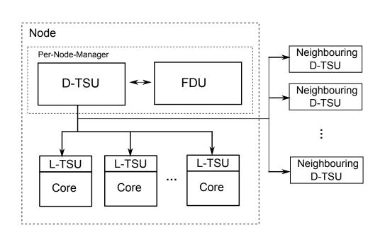
Figure 4.7: Overview of the Thread Scheduling Unit (TSU).
