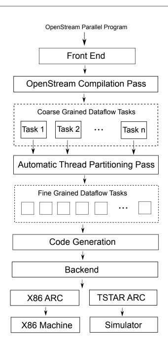
Figure 8.1: High level overview of the compilation and simulation architecture.
