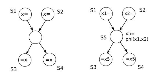
Figure 3.7: Definition and use edges in the presence of control flow.
