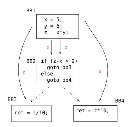
Figure 4.3: Program dependence graph of an illustrative example.
