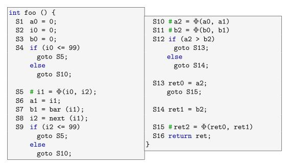
Figure 5.5: SSA representation after loop unswitching.
