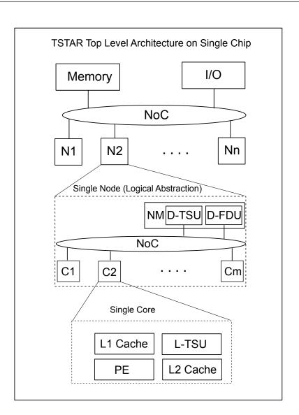
Figure 4.6: TSTAR Highlevel Architecture.
