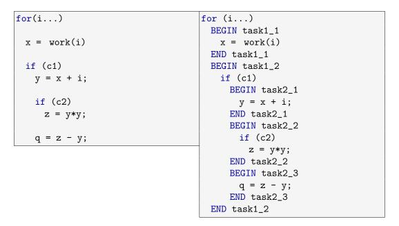
Figure 3.12: Before partitioning (left), and After partitioning (right). Loop with control dependences.
