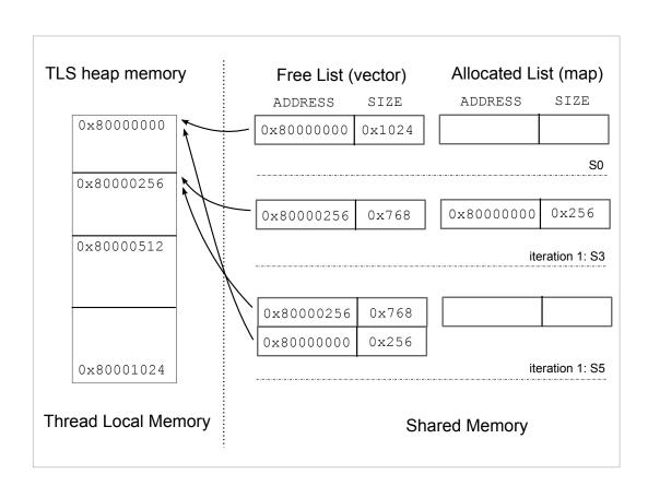
Figure 7.6: Host Space TLS Frame Memory Allocator
