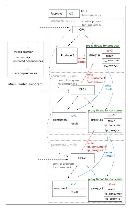
Figure 6.4: Single producer multiple consumers
