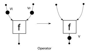
Figure 4.1: Firing rule example.
