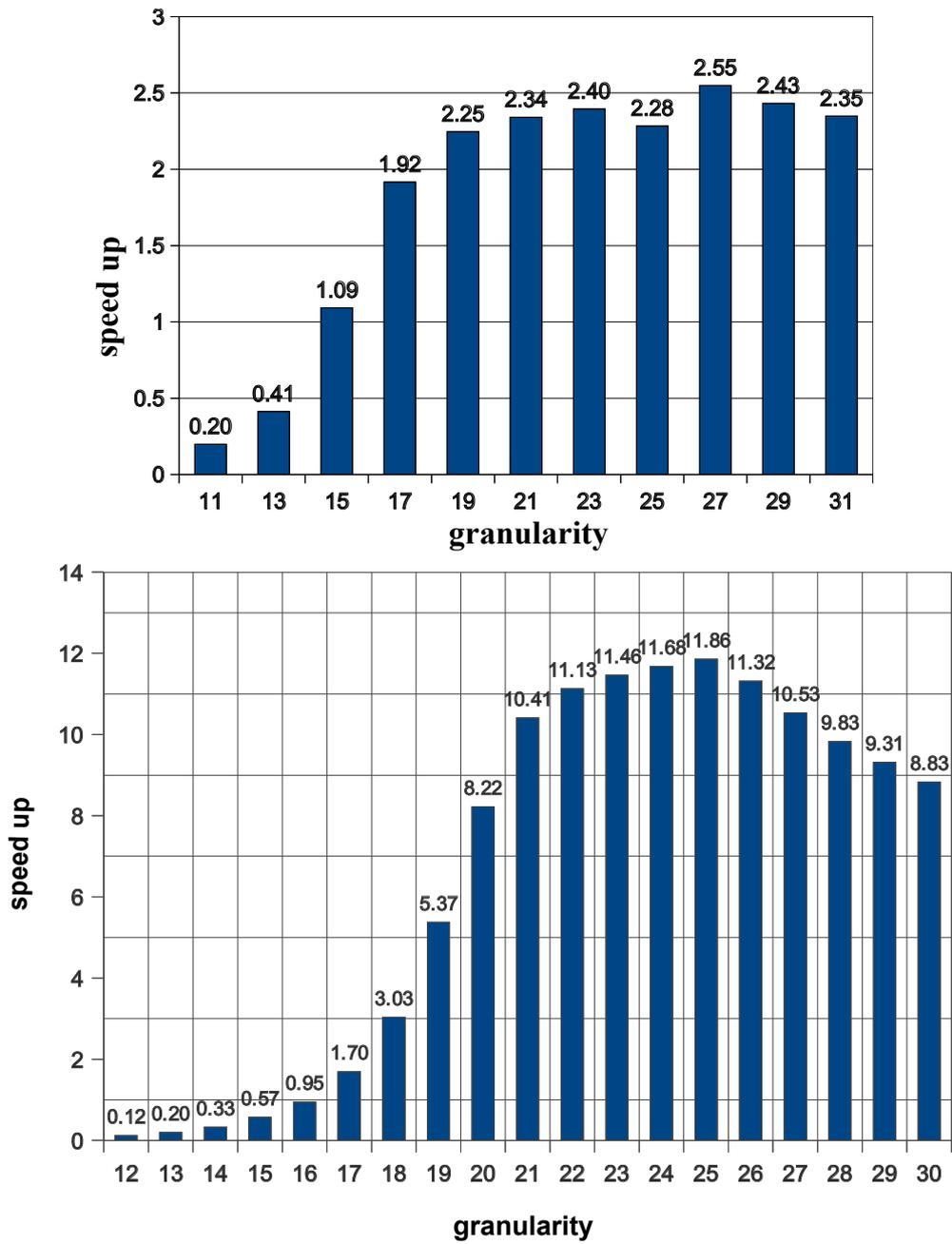
Figure 5.15: Computing the 42<sup>th</sup> Fibonacci number on 4 cores (above) and 24 cores (below).
