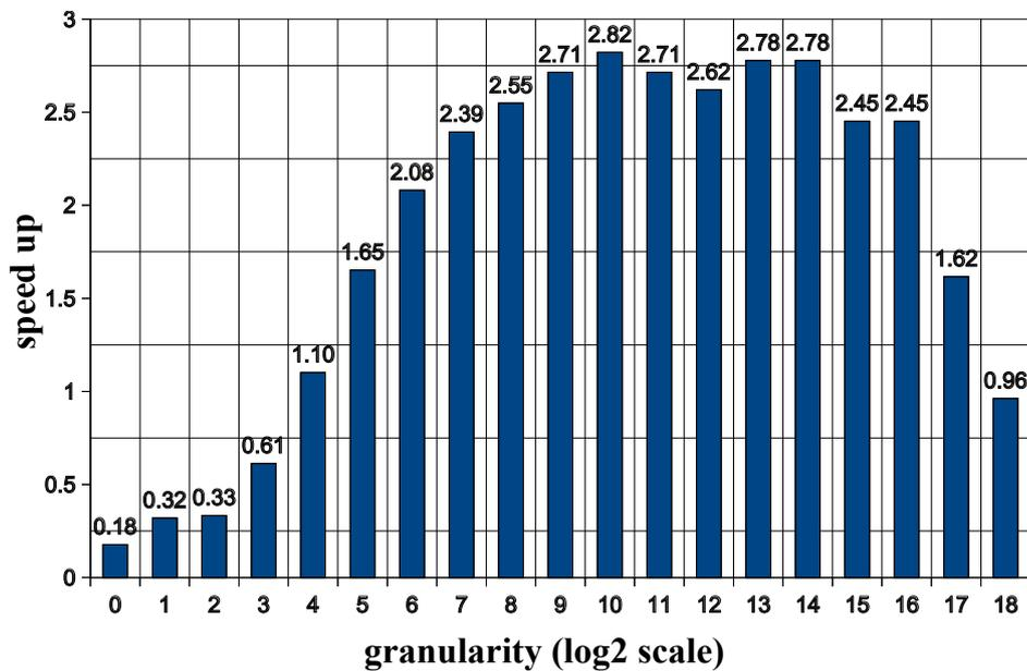
Figure 5.14: Merge Sort running on 4 cores.
