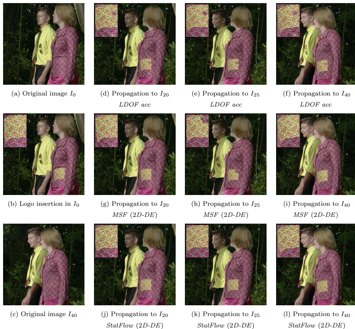
Figure 11.26: Texture insertion in I_0 and propagation up to I_{40} ( Walking-Couple-0-60 sequence). We compare: d-f) Euler integration using LDOF [BM11] elementary optical flow fields computed between consecutive frames: LFOF acc ; g-i) multi-step flow fusion (Section 11.2) using 2D-DE multi-step elementary optical flow fields: MSF(2D-DE) ; j-l) the statistical multi-step flow (Section 11.3) using 2D-DE multi-step elementary optical flow fields: StatFlow(2D-DE) .
