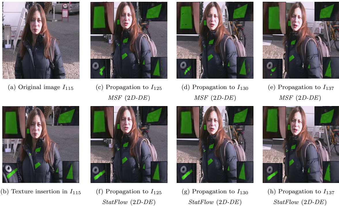
Figure 11.23: Texture insertion in I_{115} and propagation along the MPI-S1 sequence [GKT + ] up to I_{137} . We compare: c-e) multi-step flow fusion (Section 11.2) using 2D-DE multi-step elementary optical flow fields: MSF(2D-DE) ; f-h) the statistical multi-step flow method (Section 11.3) using 2D-DE multi-step elementary optical flow fields: StatFlow(2D-DE) .
