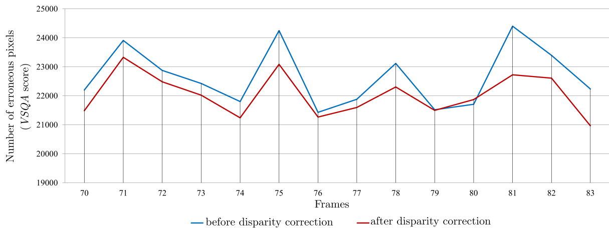
Figure 14.4: Comparison between the VSQA curves (built using VSQA scores) obtained before and after disparity correction ( Book-Arrival binocular sequence). The two reference pairs of frames used for this experiment are as follows: \{I_{69}^l, I_{69}^r\} and \{I_{84}^l, I_{84}^r\} .
