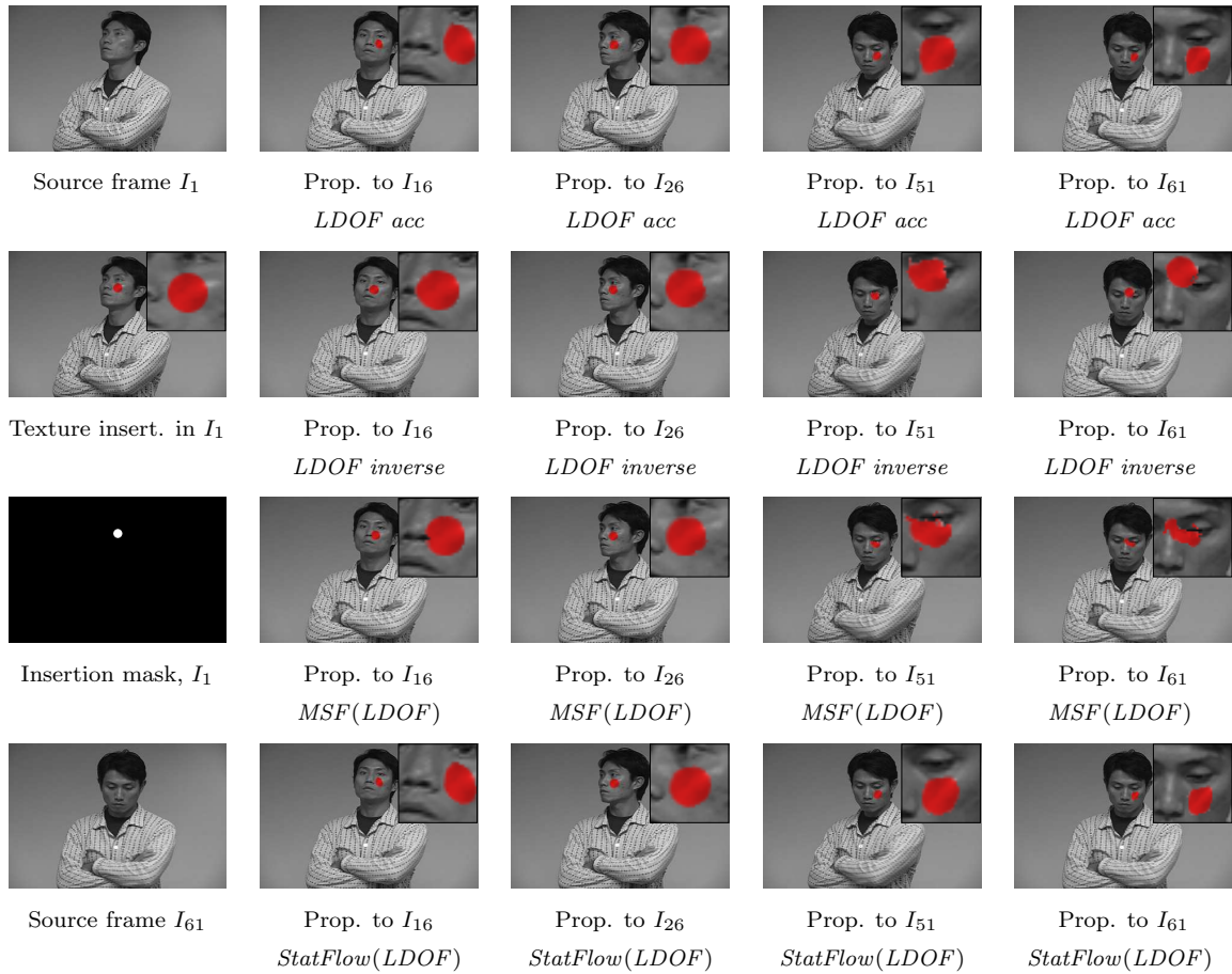
Figure 11.32: Texture insertion in I_1 and propagation up to I_{61} ( Hopkins-head sequence). We compare: Euler integration using LDOF [BM11] consecutive elementary optical flow fields: LDOF acc ; inverse integration of LDOF consecutive elementary optical flow fields: LDOF inverse ; multi-step flow fusion ( MSF ) described in Section 11.2 using LDOF multi-step elementary optical flow fields: MSF(LDOF) ; statistical multi-step flow ( StatFlow ) proposed in Section 11.3 using LDOF multi-step elementary optical flow fields: StatFlow(LDOF) .
