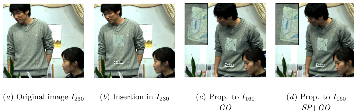
Figure 11.11: Logo insertion in I_{230} (a,b) and propagation to I_{160} ( Newspaper-2 sequence, Fig. 11.7). We compare the global optimization ( GO ) method (c) with the statistical processing ( SP ) combined to GO ( SP+GO ) (d).
