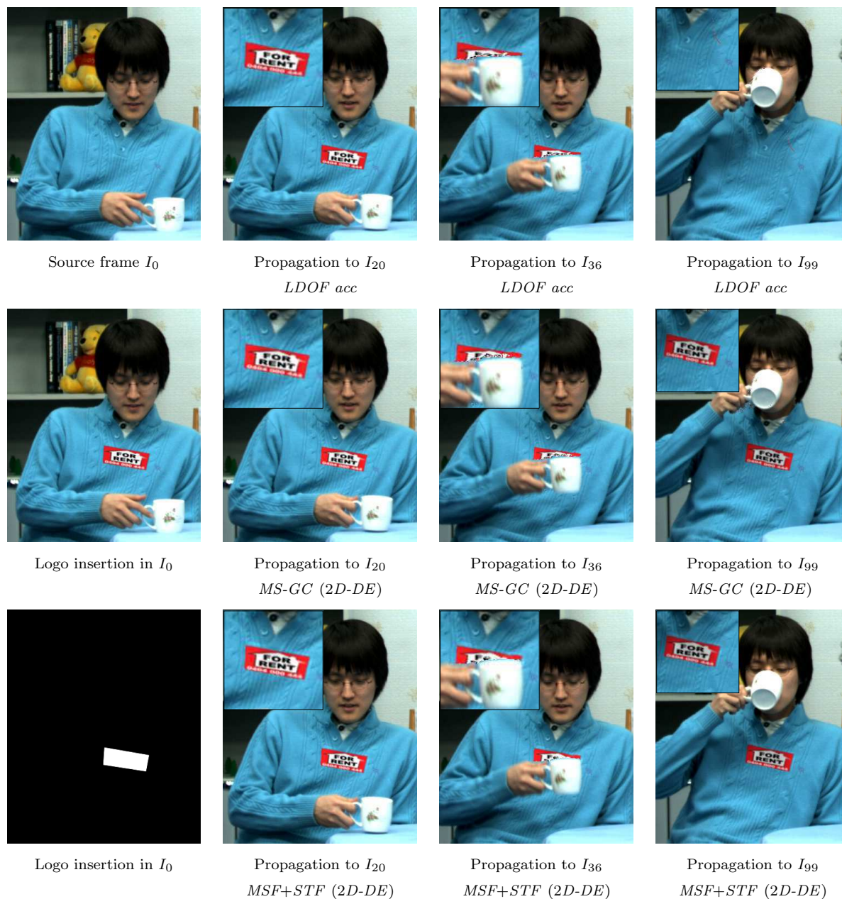
Figure 10.20: Logo insertion in I_0 and propagation up to I_{99} ( Newspaper sequence). We compare: the classic direct integration of consecutive LDOF [BM11] optical flow ( LDOF acc ); the proposed multi-step via graph-cuts approach (Section 10.1) using multi-step elementary 2D-DE optical flows [RTDC12], MS-GC (2D-DE) ; the proposed multi-step flow approach (Section 10.2) using multi-step elementary 2D-DE optical flows , MSF+STF (2D-DE) .
