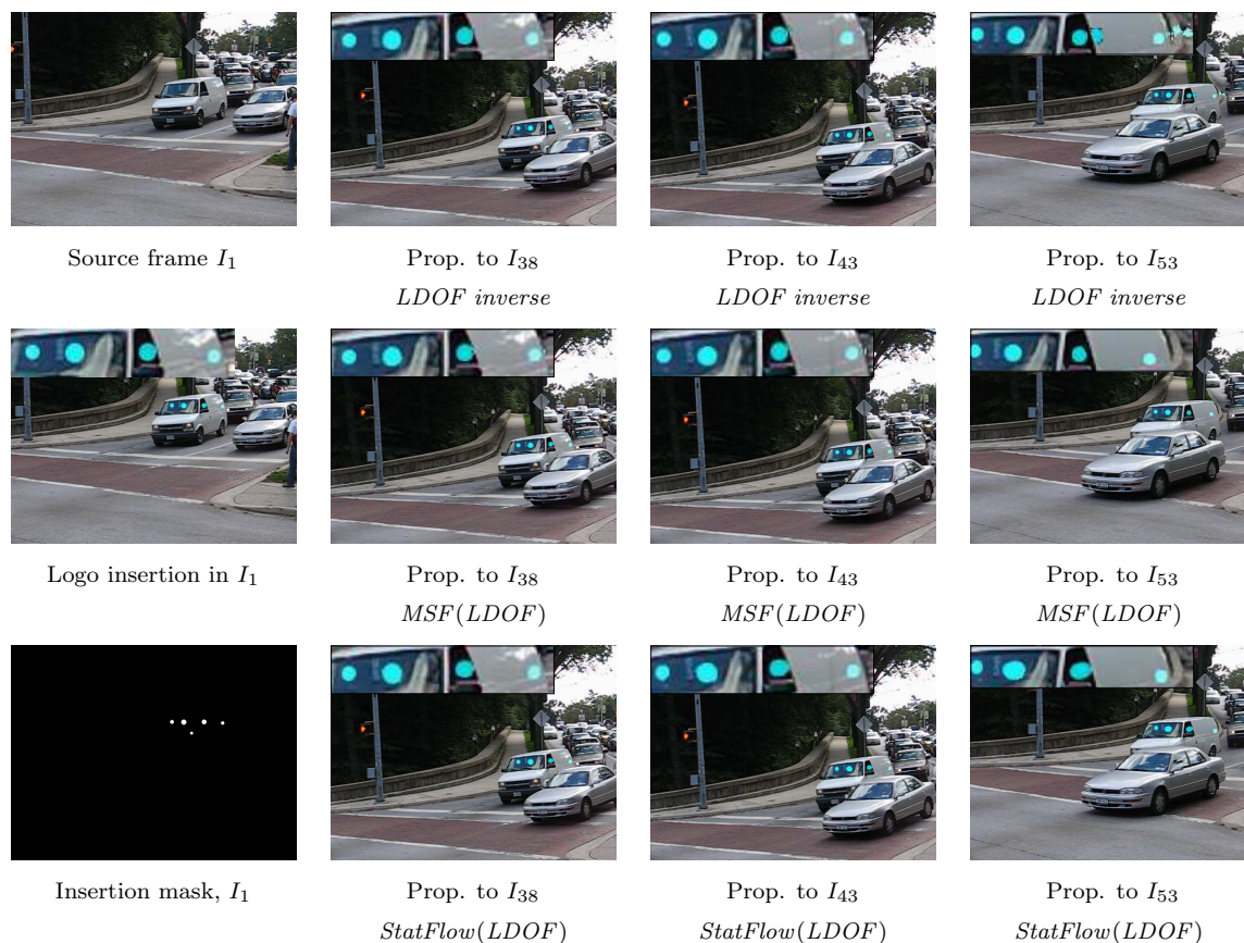
Figure 11.33: Texture insertion in I_1 and propagation up to I_{53} ( Hopkins-cars9 sequence). We compare: inverse integration of LDOF consecutive elementary optical flow fields: LDOF inverse ; multi-step flow fusion ( MSF ) described in Section 11.2 using LDOF multi-step elementary optical flow fields: MSF(LDOF) ; statistical multi-step flow ( StatFlow ) proposed in Section 11.3 using LDOF multi-step elementary optical flow fields: StatFlow(LDOF) .
