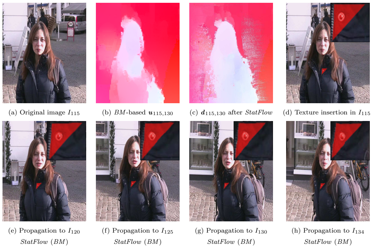
Figure 11.34: Logo insertion in I_{115} and propagation along the MPI-S1-155-175 sequence up to I_{134} with the statistical multi-step flow ( StatFlow ) method proposed in Section 11.3 using block matching ( BM ) multi-step elementary optical flow fields.
