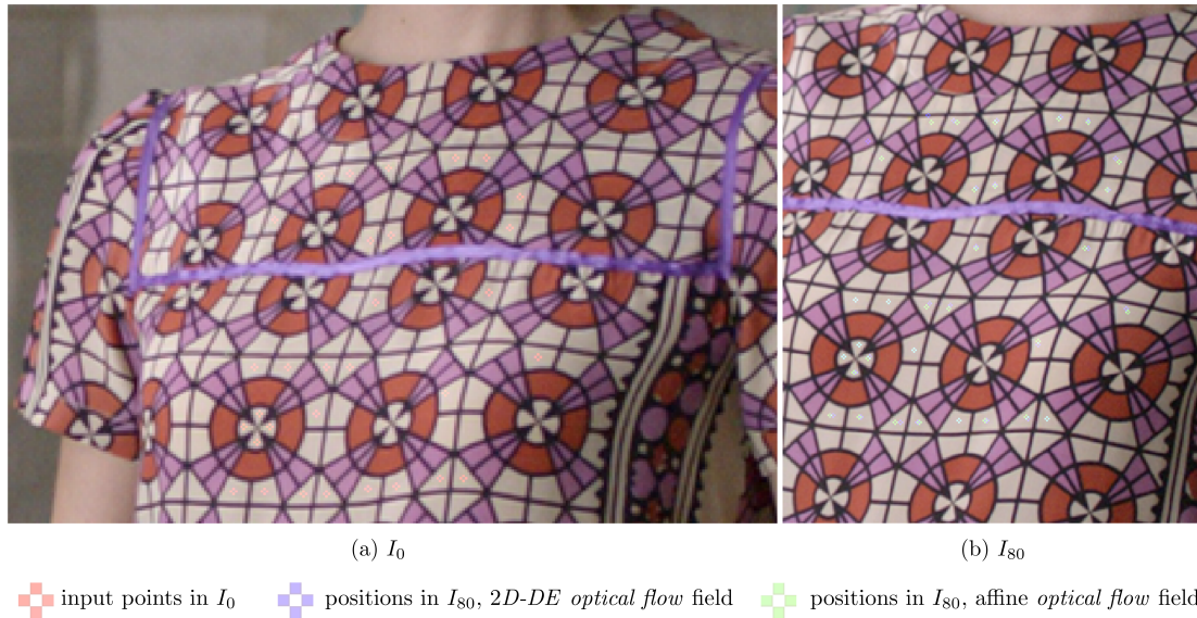
Figure 10.18: Matching results in AmeliaRetro between I_0 and I_{80} with an optical flow field computed using 2D-DE and an affine optical flow field estimated via quadtree decomposition and RANSAC algorithms. The input points (red points in (a)) are located at the center of white areas of the dress.
