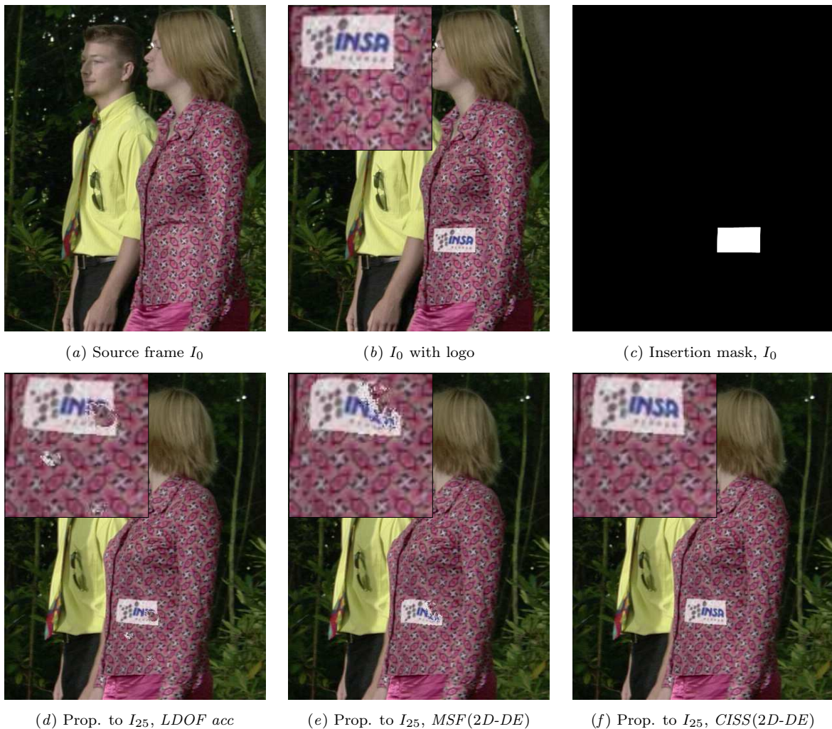
Figure 11.15: Texture insertion in I_0 and propagation in I_{25} ( Walking-Couple-0-60 sequence). We compare: Euler integration using LDOF [BM11] elementary optical flow fields computed between consecutive frames: LDOF acc ; multi-step flow fusion ( MSF ) described in Section 10.2 using 2D-DE multi-step elementary optical flow fields: MSF(2D-DE) ; the combinatorial integration followed by the statistical processing combined to the global optimization ( CISS ) using 2D-DE multi-step elementary optical flow fields: CISS(2D-DE) .
