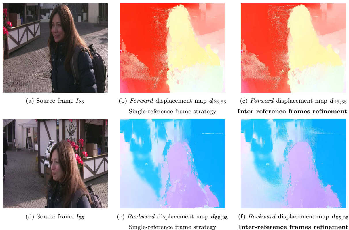
Figure 12.19: Visualization of the forward and backward inter-reference frames displacement maps ( MPI-S1-25-55 sequence). We compare: 1) a single-ref. frame strategy based on StatFlow(2D-DE) performed from I_{25} , 2) the inter-reference frames motion refinement (first step of the two-reference frames motion refinement) proposed in Section 12.3.1 and based on StatFlow(2D-DE) performed in forward from I_{25} and in backward from I_{55} .
