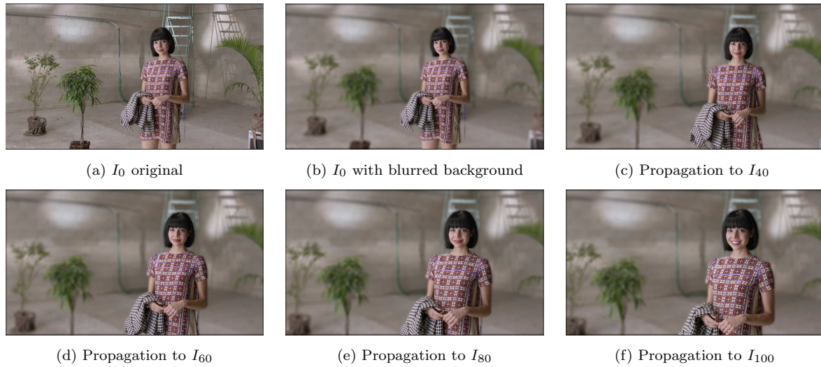
Figure 10.25: Blurring of the background of AmeliaRetro . Thanks to the segmentation labels which have been propagated through the sequence via our MSF+STF(2D-DE) long-term displacement fields, we are able to identify for each frames of the sequence the pixels which belong to the background in order to finally apply a low-pass filtering.
