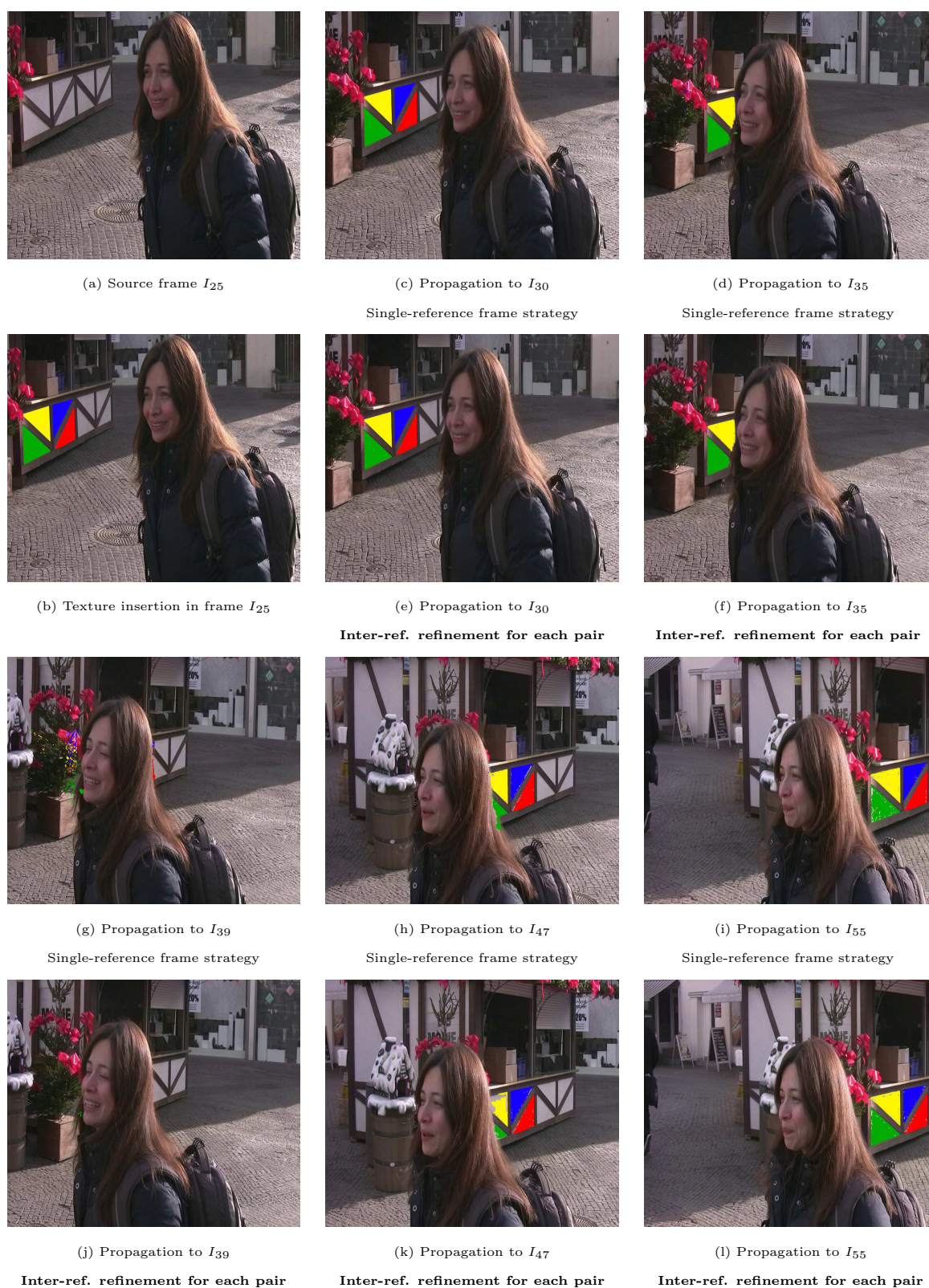
Figure 12.26: Texture insertion in I_{25} and propagation along the MPI-S1-25-55 sequence up to I_{55} . We compare: 1) the single-ref. frame strategy based on StatFlow(2D-DE) performed from I_{25} , 2) the inter-ref. refinement (Section 12.3.1) applied to each pair \{I_{ref}, I_n\} which assumes that StatFlow(2D-DE) has been applied in forward from I_{25} and in backward from each frame of the sequence.
