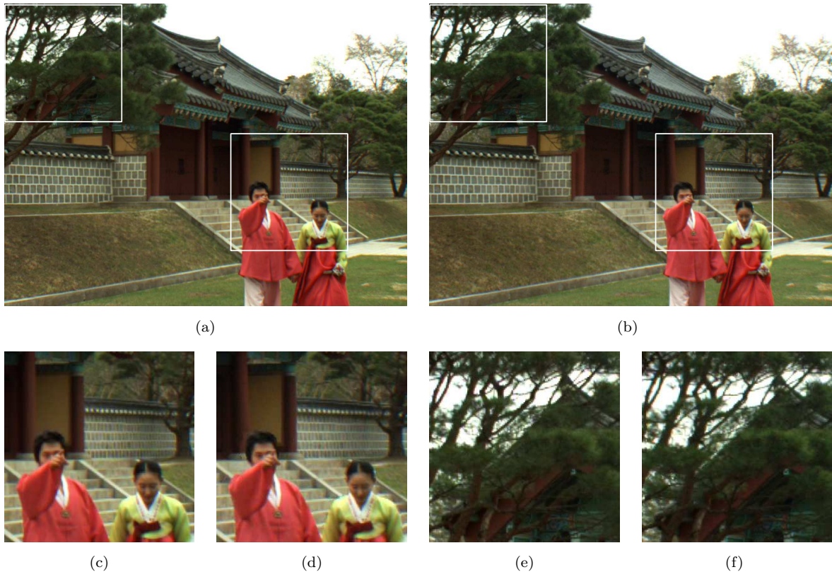
Figure 6.8: Reference (a) and synthesized (b) views with zooms on two distorted areas: (c,e) for the reference view and (d,f) for the synthesized view. The reference view is taken from the Lovebird-1 binocular sequence. The synthesized view has been created by the disparity-compensated view synthesis proposed in [RTDC12].
