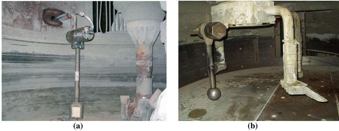
Figure 1.13 Sonde Orbiter (a) ; Sonde Viscoprobe (b)
