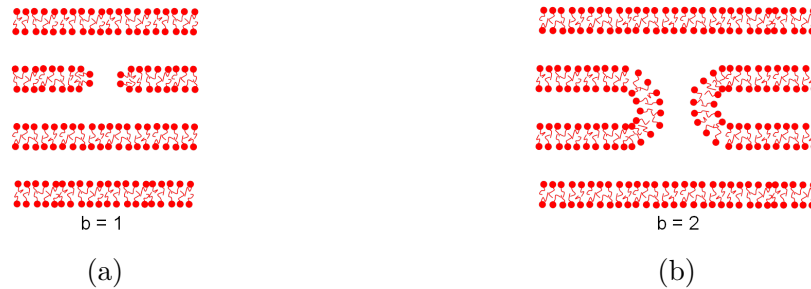
Figure 2.9: Edge dislocations of Burgers vector b = 1 (Figure a) and b = 2 (Figure b).
