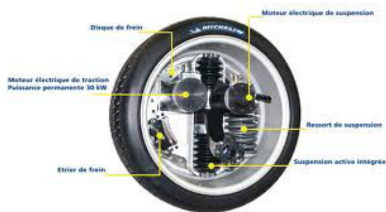
Figure 3-11 - Michelin "Active Wheel"
