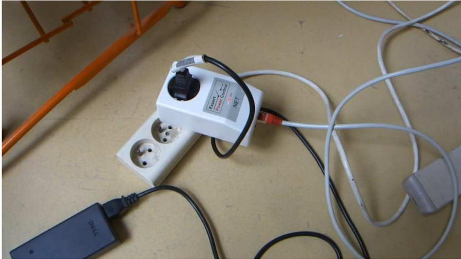
Figure 68 : prise programmable via port Ethernet
