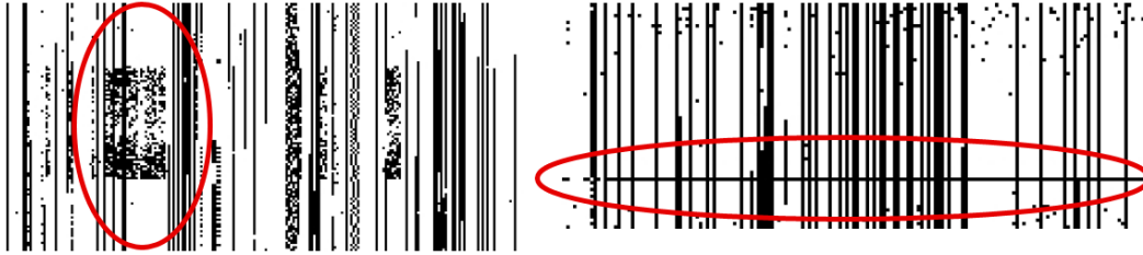
Figure 3.21: Barcode metaphor [ALGL11]: a white dot at coordinates (i, j) means that node j exists at time step i . The full dynamics is captured in a single view. We circle an outlier block of nodes (left) and an outlier time step (right).
