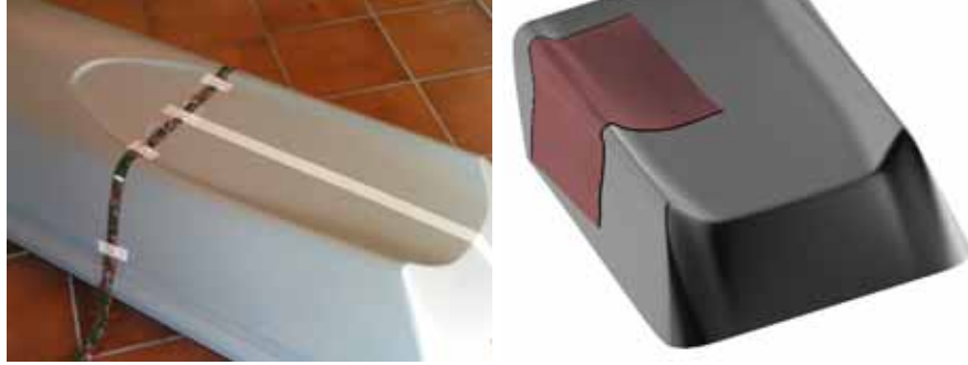
Fig. 3.15 - Reconstruction of a part of a physical surface from ribbon's data representing transversal geodesic curves.
