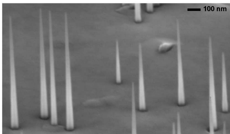
FIGURE 3.1: SEM image of ZnTe nanowires on as-grown sample
