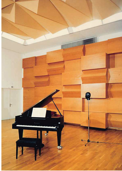
Figure B.1: Musical studio of the PTB with wooden diffusers.
