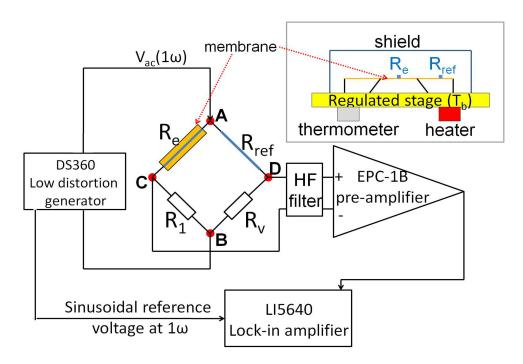
Figure 2.5: Schematic of the electrical measurement system including HF filter, preamplifier, and lock-in amplifier. A, B, C, and D represent the nodes of the Wheatstone bridge. The  $V_{3\omega}$  is measured between C and D. The transducer is referred to as  $R_e$  and the reference resistance as  $R_{ref}$ . The inset presents a schematic of the membrane fixed on the temperature regulated stage covered by the thermal copper shield.
