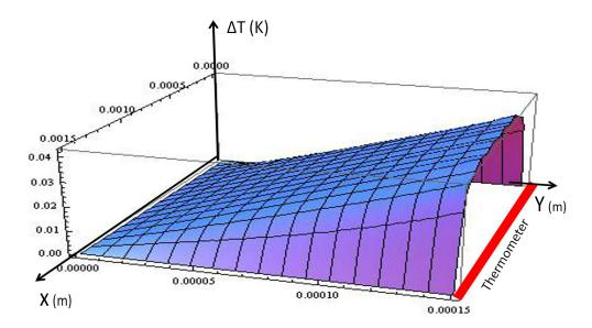
Figure 3.2: Schematic shows the steady state temperature profile on half of the membrane, at room temperature for a dissipated power of 1  $\mu$ W and thermal conductivity  $\kappa \sim$  3 W/m.K. The temperature elevation on the centre of the membrane is  $\Delta T \sim$  40 mK.
