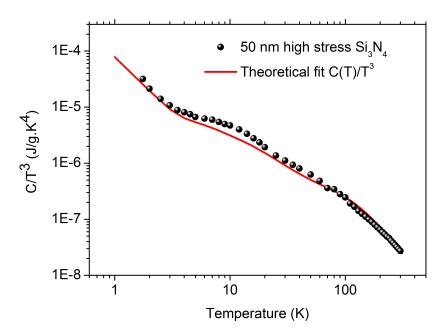
Figure 4.8: Specific heat measurement of 50 nm  $Si_3N_4$  membrane divided by  $T^3$ . The solid line is the theoretical fit.
