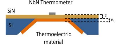
Figure 5.1: Schematic of SiN membrane shows the thermoelectric material deposited on the backside. e is the thickness of the membrane and  $e_1$  the thickness of the thermoelectric film.
