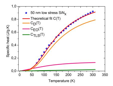
Figure 4.5: Specific heat measurement of 50 nm low stress  $SiN_x$ . The red solid line is the theoretical fit to experimental data C(T), is given by the sum of  $C_D(T)$ ,  $C_{EO}(T)$  and  $C_{TLS}(T)$ . The parameters of the fit are given in Table 4.1.
