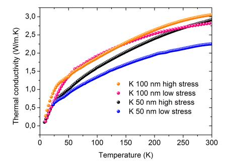
Figure 4.13: Thermal conductivity measurement of 50 nm and 100 nm thick membrane for both SiN low stress and high stress. The 100 nm curves of low stress and high stress show nearly no difference. The 50 nm curves show more difference at high temperature.
