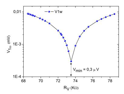
Figure 2.7:  $V_{1\omega}$  versus  $R_{\nu}$  measured between C and D. This measurement is performed at T= 150 K, with  $V_{ac} = 1$  V and f = 7.56 Hz.
