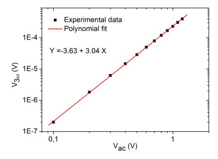
Figure 3.7:  $3\omega$  voltage measurement as a function of the voltage applied across the Wheatstone bridge  $V_{ac}$  in logarithmic scales (T = 270 K,  $R_e$  = 200 K $\Omega$ ,  $\alpha$  =0.0063 K<sup>-1</sup>). The slope of the linear fit is very close to 3 confirms the cubic behavior of the  $V_{3\omega}$  signal versus the applied voltage  $V_{ac}$ .
