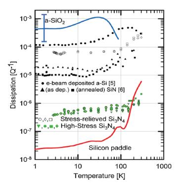
Figure 4.3: Temperature dependent internal friction measured for same high-stress LPCVD Si<sub>3</sub>N<sub>4</sub> membrane structures. This is contrasted with the behavior of *a*-SiO<sub>2</sub> (solid blue line) and single crystal Si (solid red line) [74,85].
