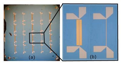
Figure 2.3: (a) Photograph shows the total chip 15x15 mm<sup>2</sup> with the 12 SiN suspended membranes and the reference transducers which are deposited on the same run onto the bulk region. (b) Photograph shows an example of two transducers used to perform the measurement of the thermal properties of SiN membranes.
