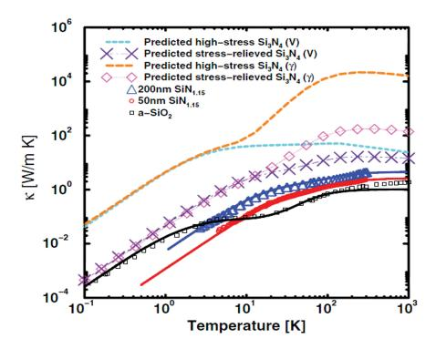
Figure 4.10:  $\kappa(T)$  vs T for amorphous SiO<sub>2</sub> and silicon nitride. Experimental data points are shown for 50- and 200-nm-thick SiN<sub>1.15</sub> and SiO<sub>2</sub>. The solid lines through the points are theoretical fits. Predictions where stress affects V or  $\gamma$  are indicated in the legend by (V) and ( $\gamma$ ), respectively [75].
