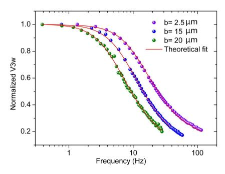
Figure 3.8:  $3\omega$  voltage measurements as function of frequency of three different samples. The measurements are performed at T=250 K, of 100 nm SiN membrane. b denotes the half width of the thermometer, where the length is the same and close to  $1500 \ \mu m$ .
