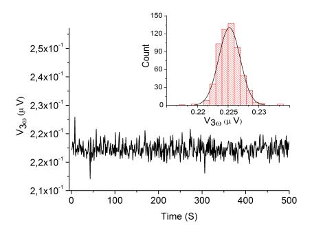
Figure 3.9: Measure of the  $3\omega$  voltage as a function of time on an 50 nm thick SiN membrane. The inset shows the signal distribution. The full width at half maximum corresponds to the noise of the measurement. In this case, the noise is evaluated to be around  $40 \text{ nV}/\sqrt{\text{Hz}}$ .
