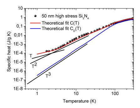
Figure 4.7: Specific heat measurement of 50 nm  $Si_3N_4$  membrane from low temperature up to room temperature. The solid blue and red lines show theoretical predictions according to Debye's model and the model given by Eq. 4.31 respectively.
