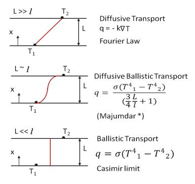
Figure 1.7: Schematic diagram showing qualitatively the steady-state temperature profiles under diffusive and ballistic phonon transport. Diffusive-Ballistic model of transport is given by Majumdar [47]
