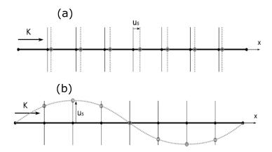
Figure 1.2: Schematics showing the vibration of atoms inside a lattice as function of the wave polarization (a) longitudinal polarization, (b) transverse polarization.
