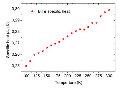
Figure 5.3: Specific heat of 200 nm thick Bi<sub>2</sub>Te<sub>3</sub> film as a function of temperature.
