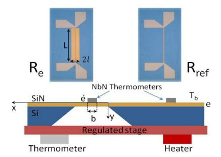
Figure 3.3: Photograph of the two NbN thermometers deposited on the membrane and on the bulk region; below, the schematic of the measurement device installed on the controlled temperature stage.
