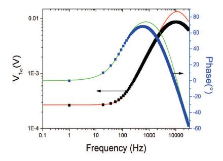
Figure 2.9: Absolute value and phase of  $V_{1\omega}$  signal as a function of the frequency and their respecting fits (solid lines) using the following parameters:  $V_{ac}^{rms} = 0.06 \text{ V}$ ,  $R_v = 70.5 \text{ K}\Omega$ ,  $R_e = 267.81 \text{ K}\Omega$   $R_{ref} = 390.77 \text{ K}\Omega$ ,  $C_3' = 185 \text{ pF}$ , and  $C_4' = 450 \text{ pF}$ .
