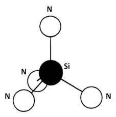
Figure 1.8: Schematic of microscopic structure of silicon nitride.
