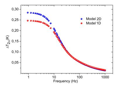
Figure 3.6: Amplitude of temperature oscillation at  $2\omega$  calculated using the 1-dimensional and 2-dimensional models. These curves are plotted using theoretical formulas of the two models and with the same fixed parameters.
