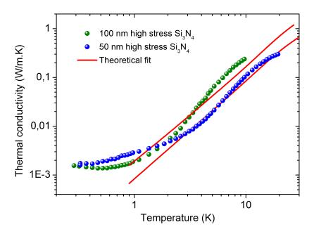
Figure 4.16: Thermal conductivity measurement of 50 nm and 100 nm high stress membrane at low temperature 300 mK < T < 300 K, along with the theoretical fits.
