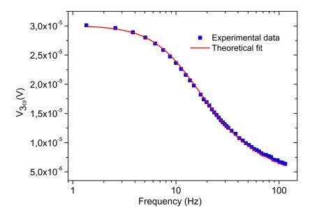
Figure 3.4:  $3\omega$  voltage measurement as function of frequency of the heater current. Experimental data agree well with the theoretical model. This measurement is performed at T = 250 K for a membrane 100 nm thick, the extracted values from the fit are  $\kappa = 3.19$  W/m.K and c = 0.68 J/g.K.
