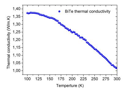
Figure 5.2: Thermal conductivity of 200 nm thick Bi<sub>2</sub>Te<sub>3</sub> film as a function of temperature.
